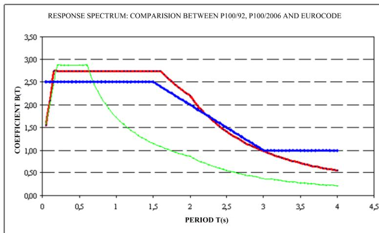
**Figure 2.** Comparison between response spectra of Bucharest given by P100-92 (bleu), P100\_1/2006 (red) and Eurocode 8 (green)
