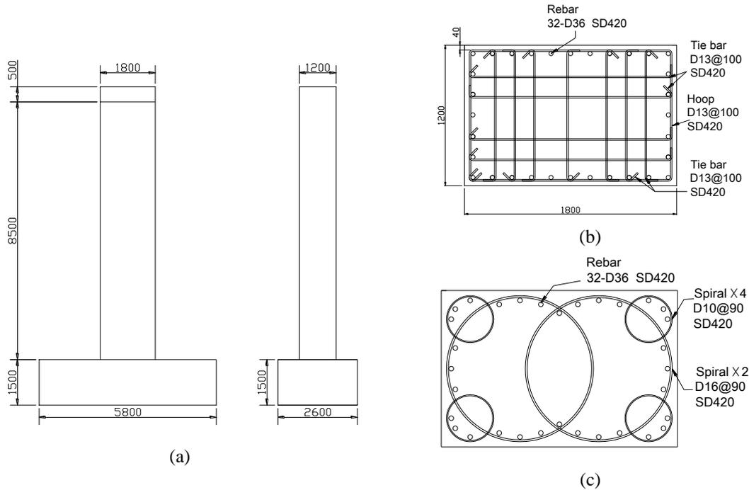
**Figure 1.** Design details of specimen (a) side view of the specimens (b) design details of the conventional column (c) design details of the proposed multi-spiral stirrup column
