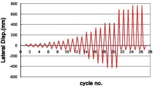
**Figure 5.** Loading protocol for the cyclic loading test
