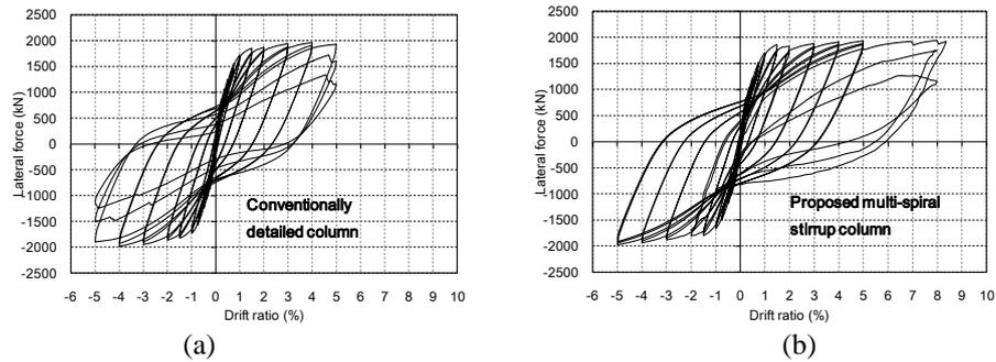
**Figure 7.** Experimental results (a) conventionally detailed column (b) proposed columns
