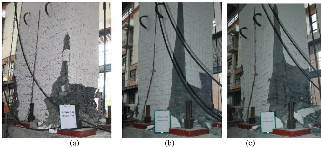
**Figure 8.** Failure photos for (a) the conventional column after drift ratio 5% (b) the proposed column after drift ratio 5% (c) the proposed column after drift ratio 8%
