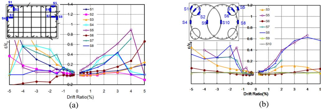
**Figure 12.** Strain ratio on the lateral reinforcements at the location 10cm above the foundation: (a) conventional column (b) proposed column
