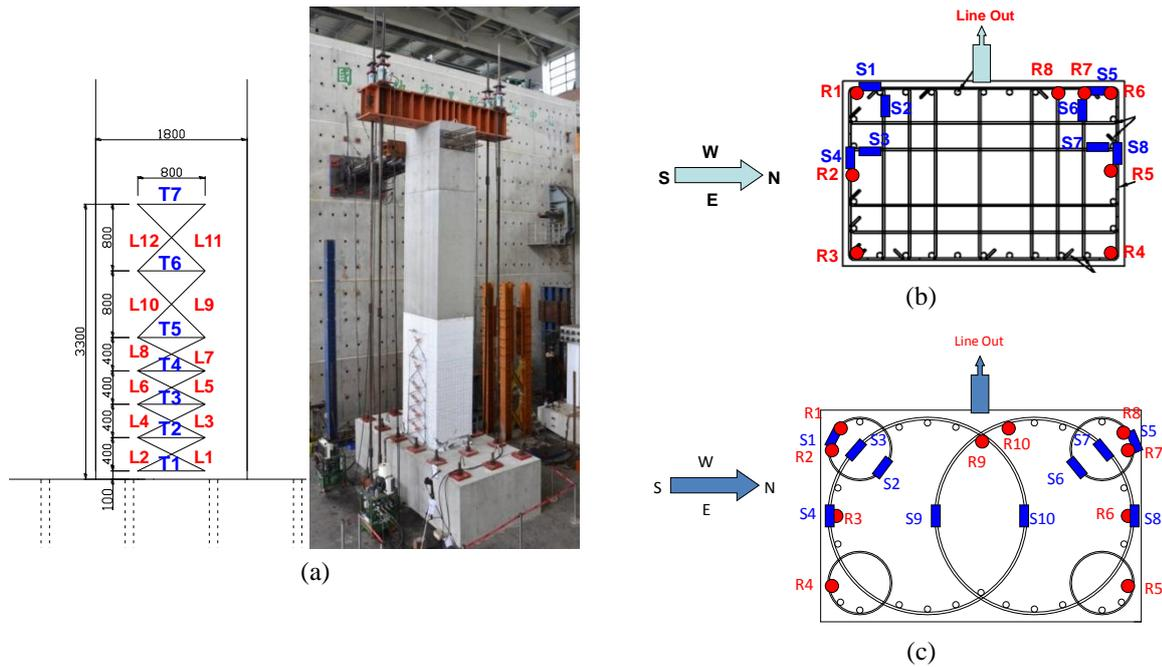
**Figure 6.** Instrumentation arrangement (a) tiltmeters and LVDT displacement gauges; (b) arrangement of strain gauge for the conventionally detailed columns; (c) arrangement of strain gaus for the proposed column
