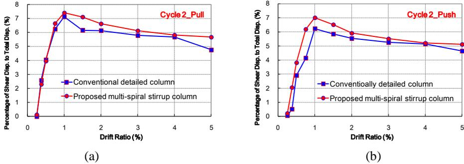
**Figure 11.** Percentage of shear displacement to the total displacement for the second cycle of cyclic loading which was applied along: (a) the south direction (pull); (b) the north direction (push)
