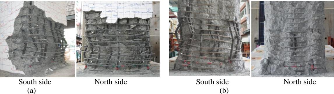
Figure 9. Comparison of failure mode (a) conventional column for drift ratio 5% (b) proposed column for drift ratio 8%
