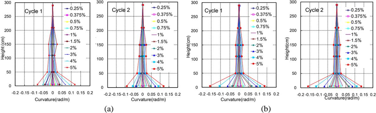
Figure 10. Curvature distributions for different drift ratios (a) conventional column (b) proposed column
