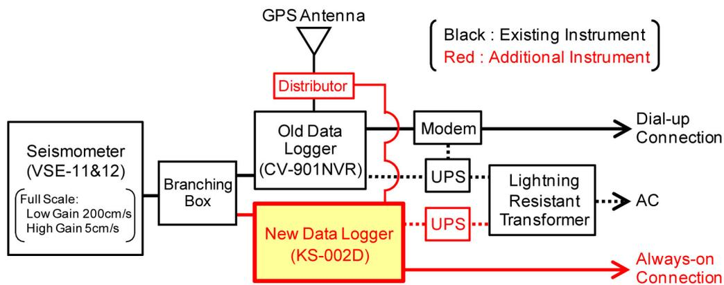
Figure 2. Basic configuration of new strong motion observation system.
