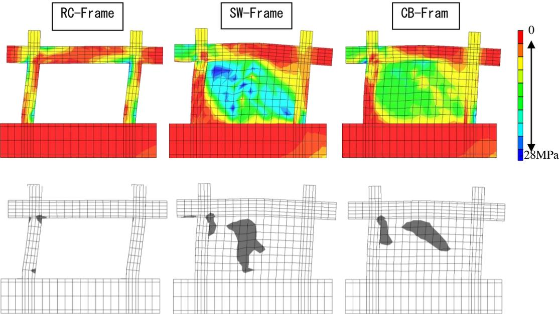
Figure 8. Concrete compressive stress contour and crushing condition
