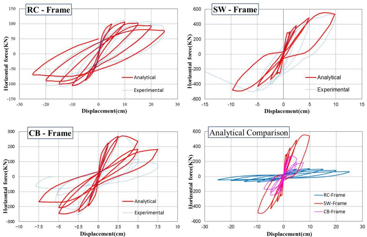
Figure 7. Relationship between story shear force and story displacement
