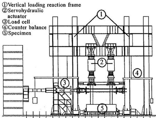
Figure 4. Experiment test setup
