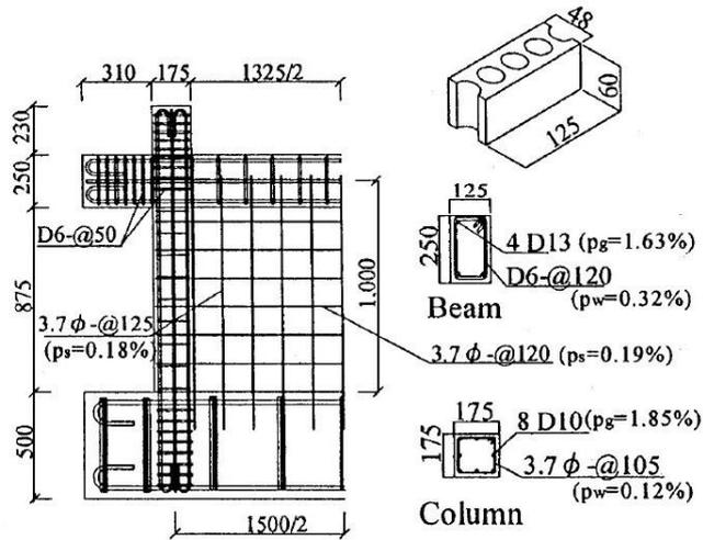
Figure 2. Details of CB-Frame specimen
