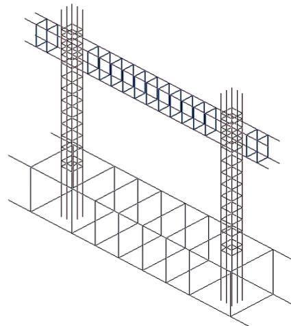
b) Rebar element (truss)
