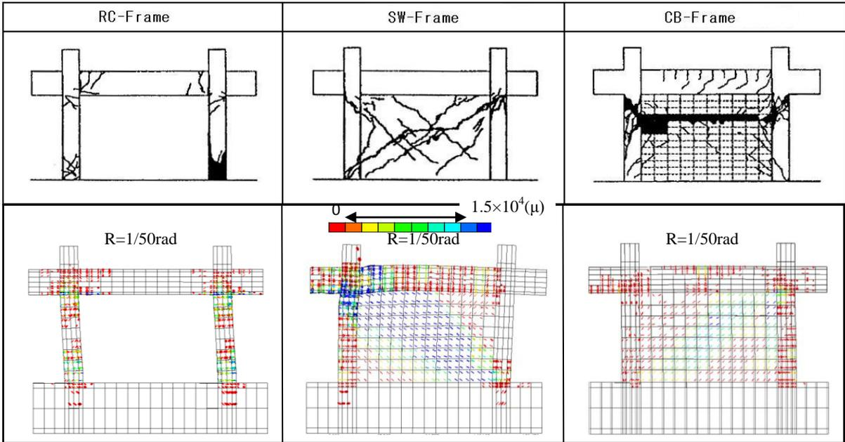
Figure 9. Comparing of Crack patterns
