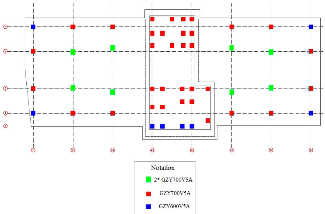
**Figure 4.2.** Rubber bearing installation scheme (real building)
