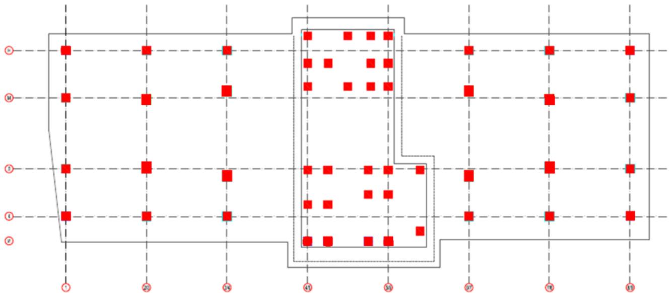
**Figure 4.3.** Rubber bearing installation scheme (scale model)
