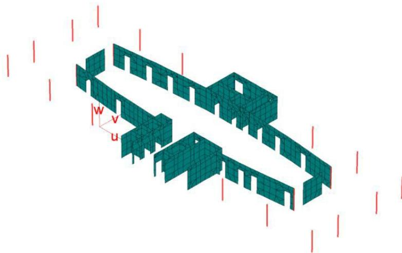
**Figure 4.1.** The layout of vertical bearing elements on the typical floor
