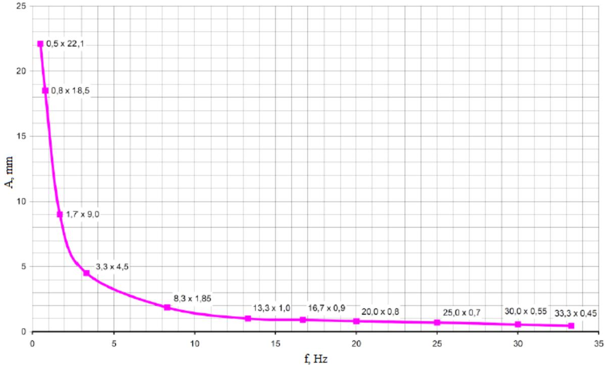
**Figure 2.2.** Schedule of permissible values of the amplitudes and frequencies for the vibroplatform EP-100
