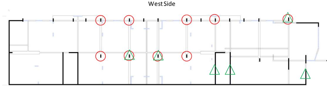
**Figure 8.** Walls of the basements with combined axial load and bending moment D/C ratios > 1.0 (red circles) and with shear stress beyond ACI limit (green triangles)
