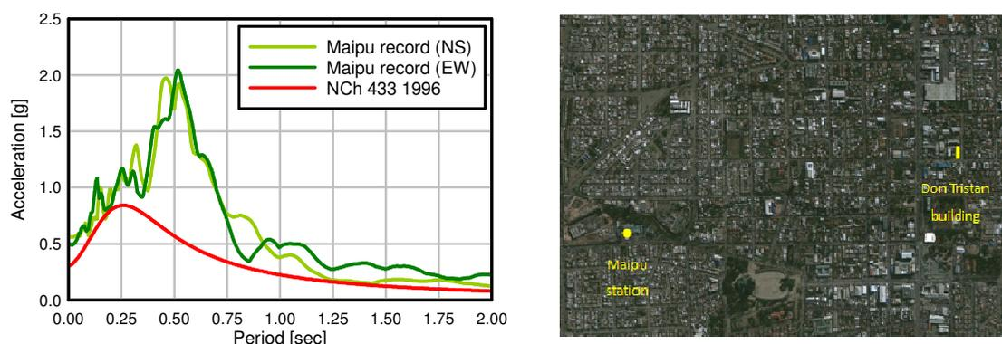
**Figure 11.** (left) Comparison between pseudo-acceleration response spectra and Code design spectra for 5% damping and (right) aerial view of the Maipú area
