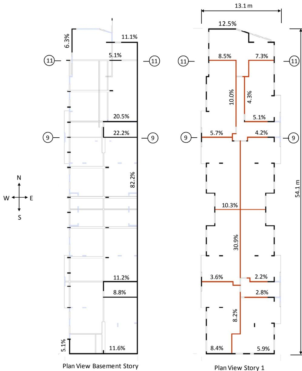
**Figure 1.** Plan view of basement and story, and percentage of story shear taken by longitudinal and transversal walls. RC elements are shown in black and CM elements in red.
