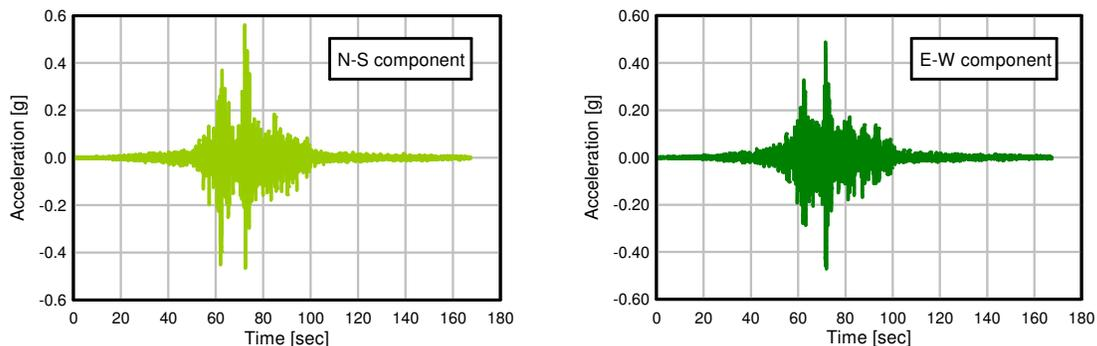
**Figure 10.** Ground acceleration histories recorded at the Maipu station during the 2010 Chile earthquake
