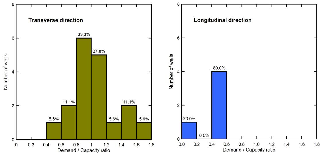
**Figure 7.**  $D/C$  ratio histogram for combined axial load and bending moment for basement walls
