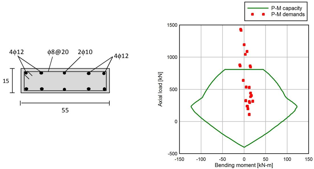
**Figure 6.** Typical detailing of 55 x 15 cm walls and confined concrete at the stirrups level (left) and interaction diagram of 55x15 cm wall in the basement of axis 9 (right)
