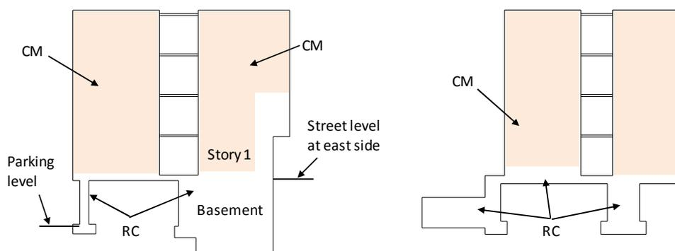
**Figure 2.** Vertical irregularity in elevation of axis 9 (left) and 11 (right)
