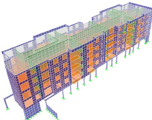
**Figure 5.** Finite element model of the building (from the west side)
