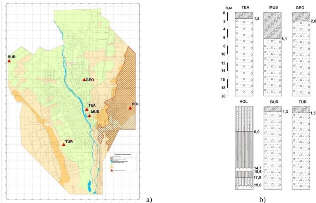
**Figure 4.** Location of seismic stations on the territory of Vladikavkaz city on engineering-geological map (a) Ground conditions of seismic stations (b)
