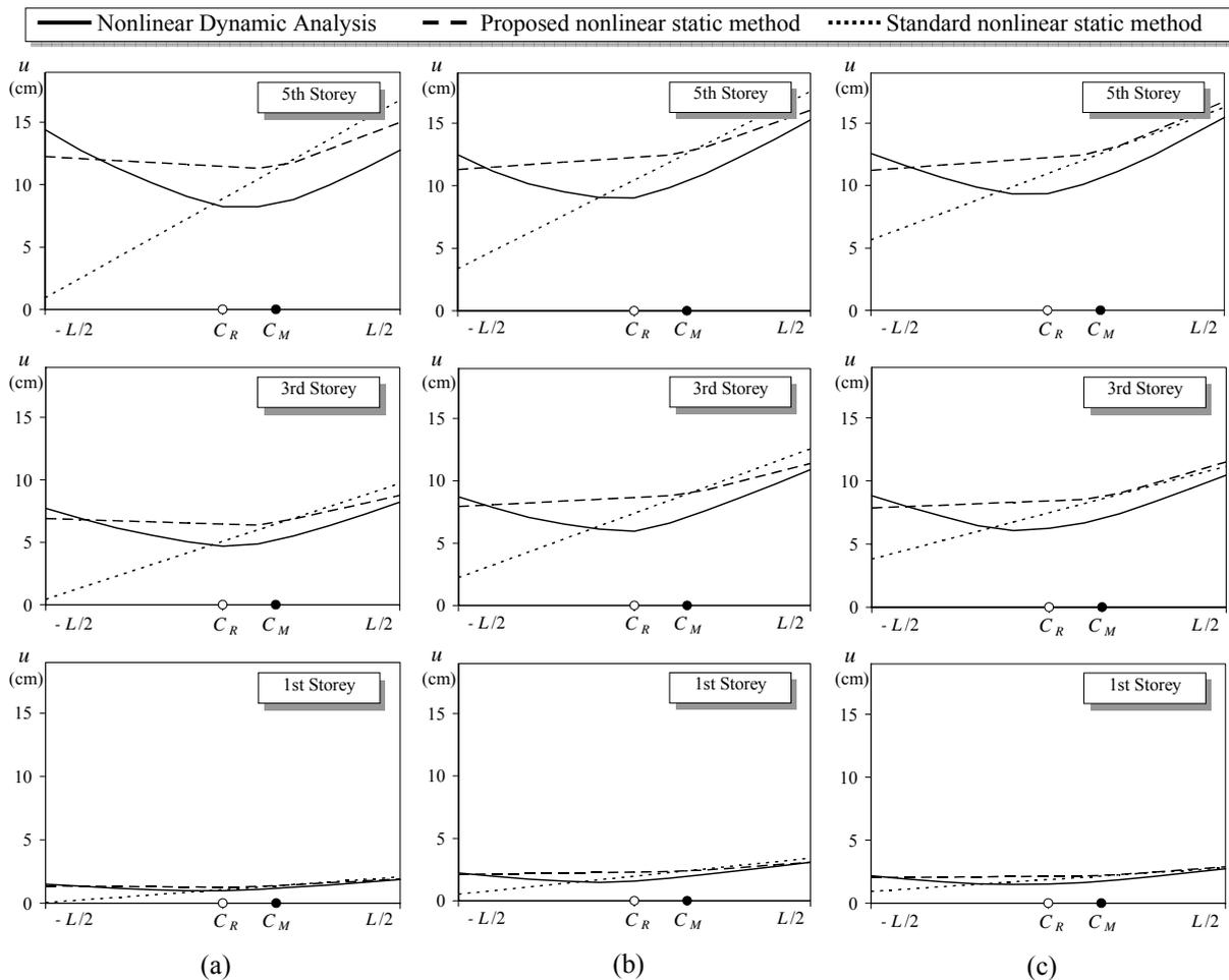
**Figure 3.** Displacements of the analysed buildings: (a) GL-H structure, (b) SR1-H structure, (c) SR2-H structure
