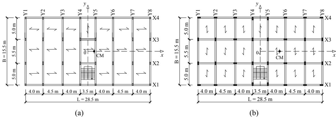
**Figure 2.** Plan layout of the analysed buildings: (a) GL structures; (b) SR structures
