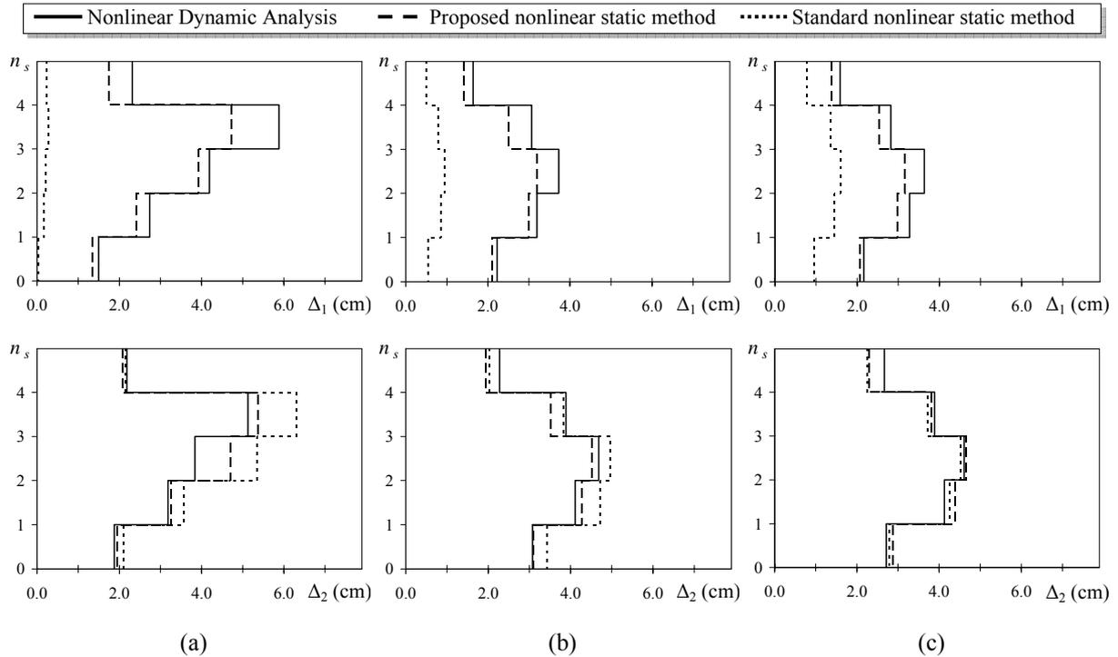
**Figure 4.** Storey drifts of the analysed buildings: (a) GL-H structure, (b) SR1-H structure, (c) SR2-H structure
