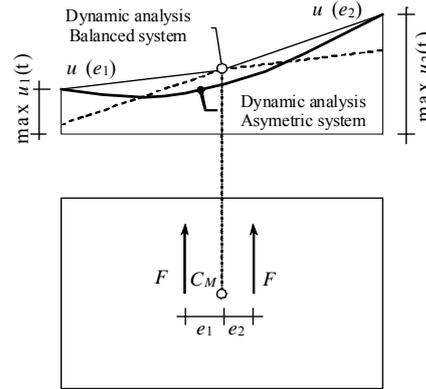
**Figure 1.** Maximum dynamic displacements vs. displacements determined by the nonlinear static method with corrective eccentricities
