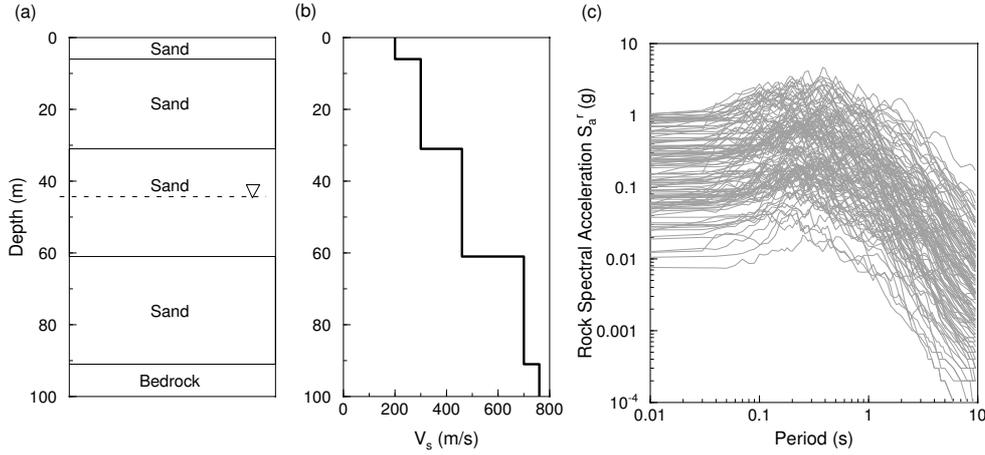
**Figure 2.1.** Site Stratigraphy, shear-wave velocity profile (after Kottke, 2006) and acceleration response spectra of the 120 rock records used in the ground response analyses
