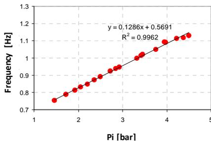
**Figure 2.4.** SDF system frequency variation
