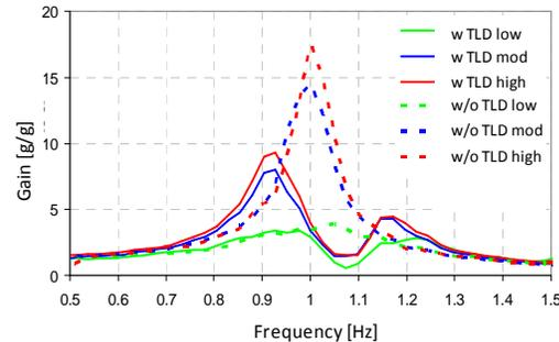
**Figure 4.4.** FRF for SDF structures with deep TLDs
