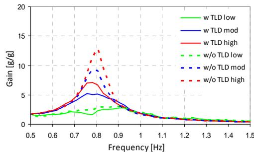
**Figure 4.3.** FRF for SDF structures with shallow TLDs
