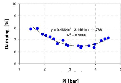
**Figure 2.5.** SDF system damping variation
