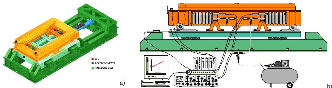
**Figure 2.2.** Instrumentation placed in the transmission structure: a) Perspective of the testing device and b) detail with connection to acquisition system and pneumatic circuit
