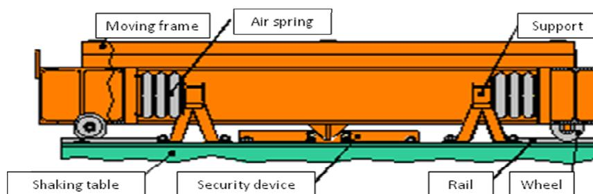
**Figure 2.1.** Testing device: SDF transmission structure
