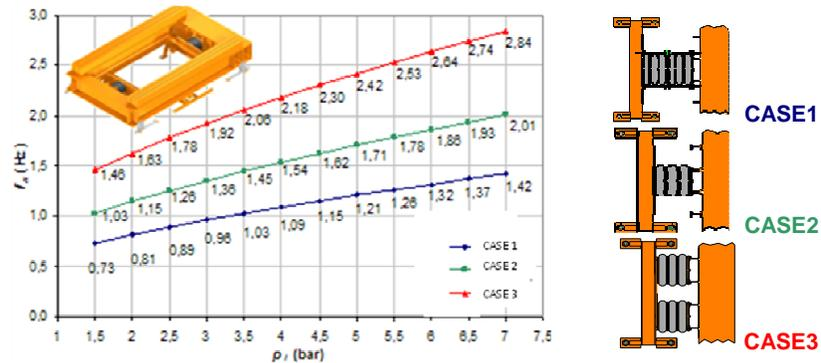
**Figure 2.3.** Frequencies for different air spring configurations, adapted from [Morais et. al., 2010]
