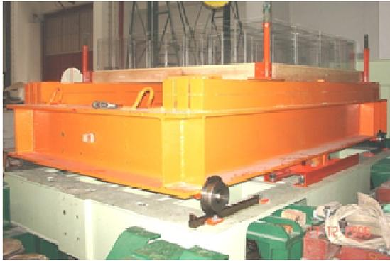
**Figure 4.1.** Set of rectangular TLDs placed on SDF reference structure
