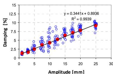
**Figure 3.5.** Damping variation in shallow TLD
