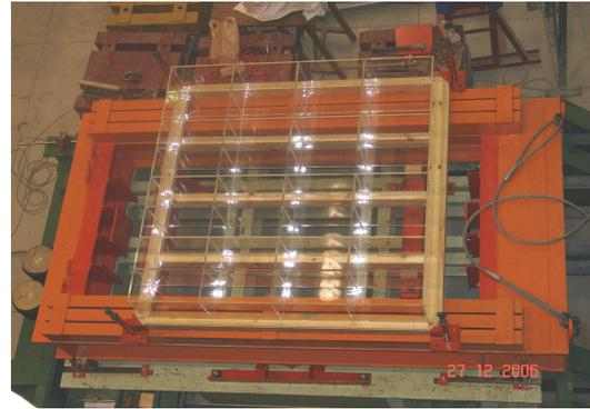
**Figure 4.2.** View from the top of the set of rectangular TLDs placed on SDF reference structure
