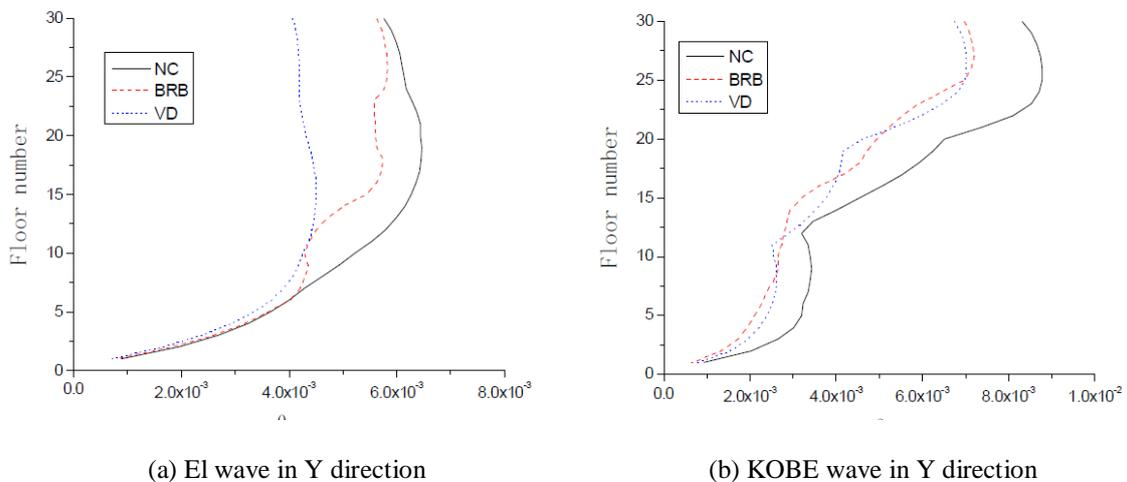
**Fig. 3.** Inter-story displacement angle of structures
