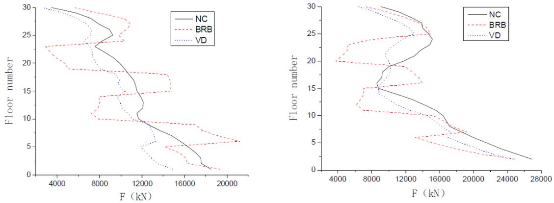
**Fig. 4.** Story shear force of structures
