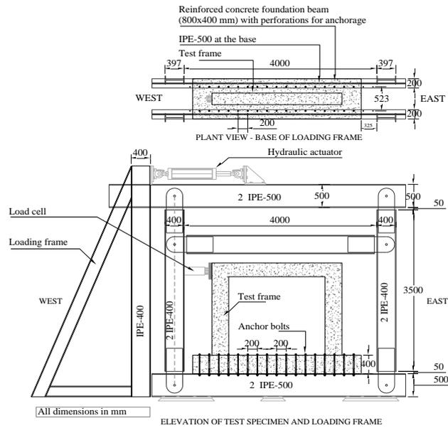
Figure 3.1. General details of loading set-up
