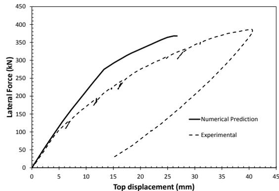
**Figure 5.2.** Numerical and experimental capacity curve
