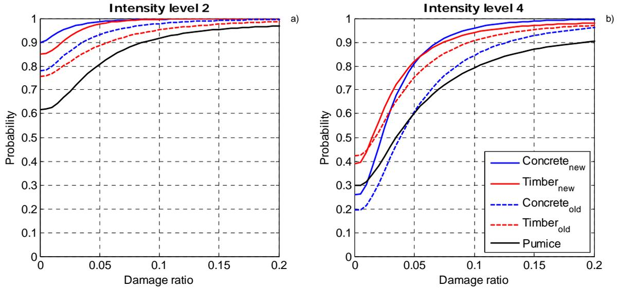
**Figure 3.** Comparison of probability functions for damage ratios of the building classes for intensity levels 3 & 4.
