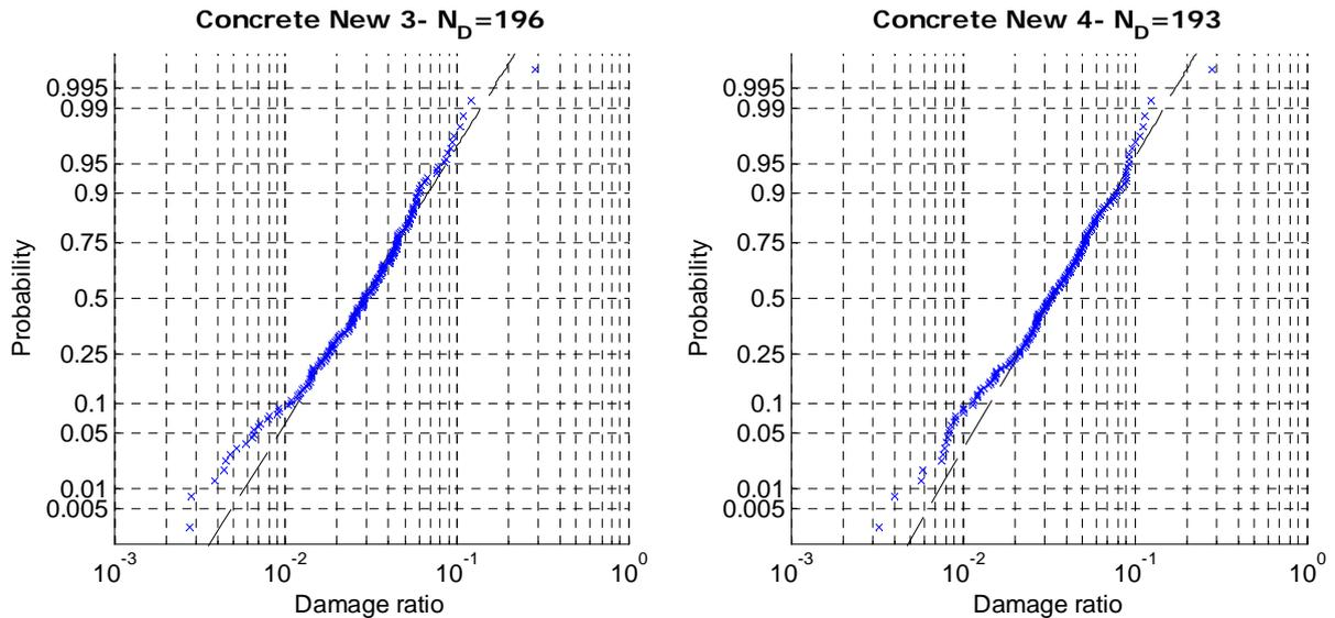
**Figure 2.** Goodness-of-fit of the damage data for the concrete<sub>new</sub> buildings to the lognormal probability function for: a) intensity levels 3, and b) intensity level 4 ( $N_D$  denotes number of damaged buildings in each case).
