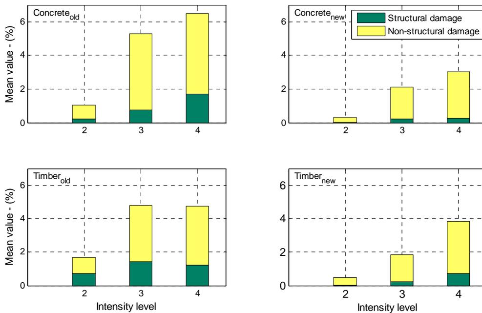
**Figure 5.** Division between structural and non-structural damage.
