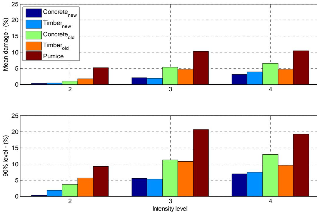
**Figure 4.** Mean damage and 90% confidence level damage for different building classes and intensity classes.
