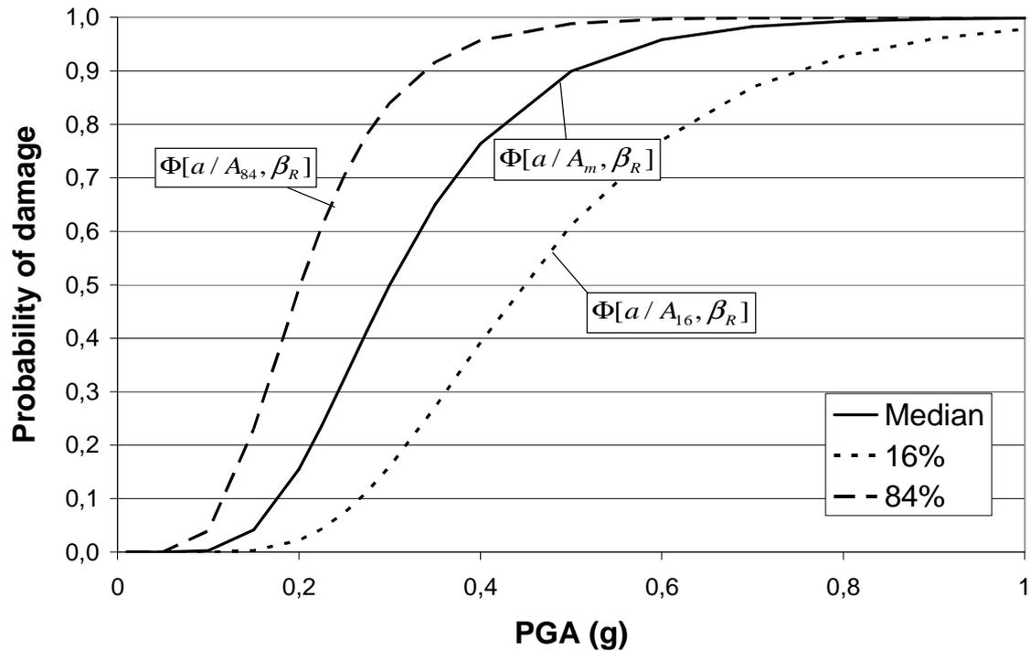
**Figure 2.** Example of lognormal fragility curves for a given damage level and for three different confidence levels
