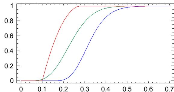
**Figure 11.** Fragility curves of central piers of Second Bridge. Seismic scenarios 1, 2 and 4
