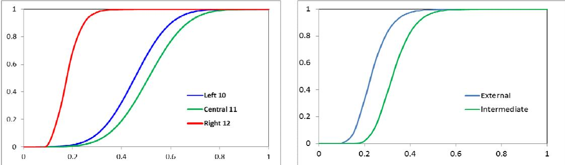
Figure 13. Fragility curves of elements of bridges with previous damage. Seismic scenario 1
