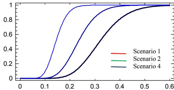
**Figure 9.** Fragility curve of the left pier of Motín de Oro Bridge. Seismic scenarios 1,2 and 4
