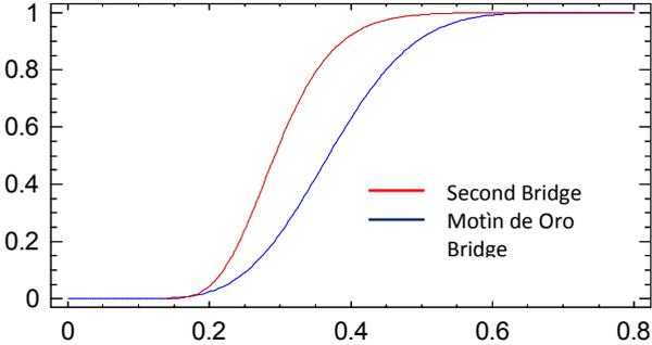
Figure 12. Fragility curves of bridges. Seismic scenario 1
