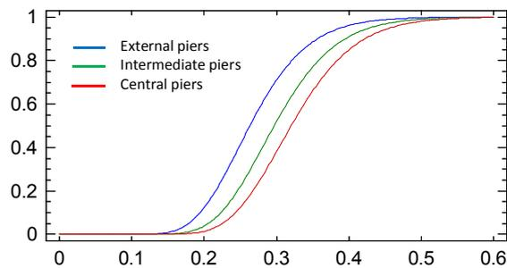
**Figure 10.** Fragility curve of piers groups of Second Bridge. Seismic scenarios 1
