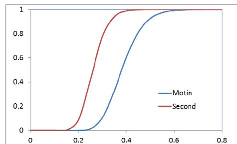
**Figure 14.** Fragility curves of bridges with previous damage. Seismic scenario 1
