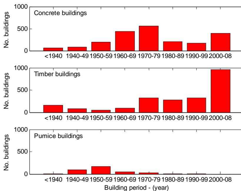
**Figure 3.1.** Age distribution of low-rise, concrete, timber and pumice buildings, in the Ölfus region.
