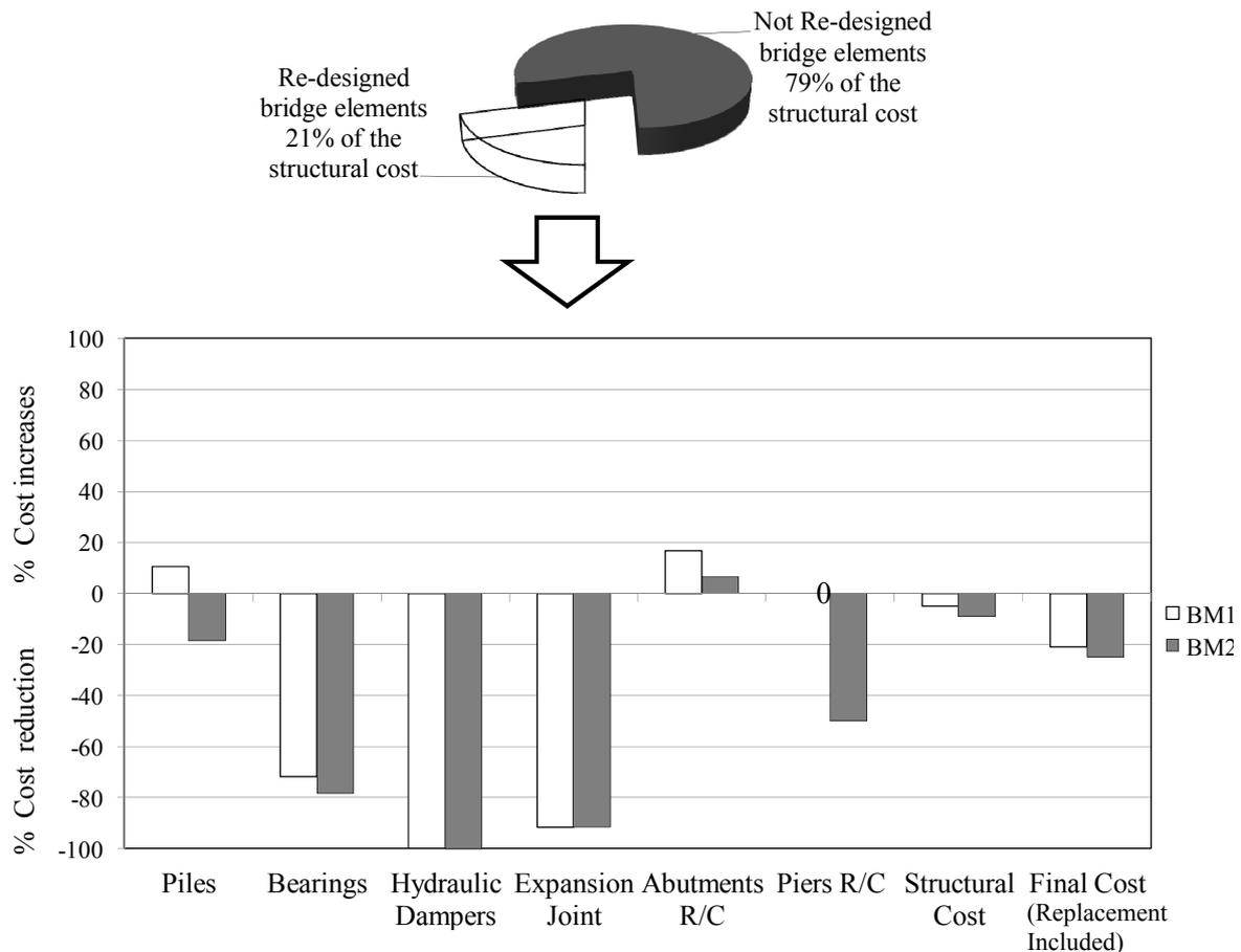
**Figure 8.** Cost sharing, the percentage cost alterations of the re-designed structural elements in the re-designed bridge systems and the percentage cost reduction of the structural and final cost of the 1<sup>st</sup> and 2<sup>nd</sup> re-designed bridge (BM<sub>1</sub> and BM<sub>2</sub>)
