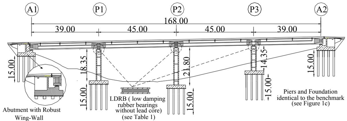
**Figure 4.** Longitudinal section of the first bridge design scheme
