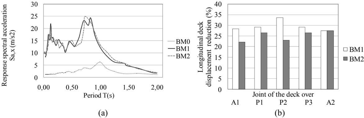
**Figure 7.** (a)The deck pseudo-accelerations longitudinal response spectra of benchmark bridge BM<sub>0</sub>, 1<sup>st</sup> re-designed BM<sub>1</sub> and 2<sup>nd</sup> re-designed BM<sub>2</sub>, (b) The percentage reduction in the longitudinal seismic displacements of the deck
