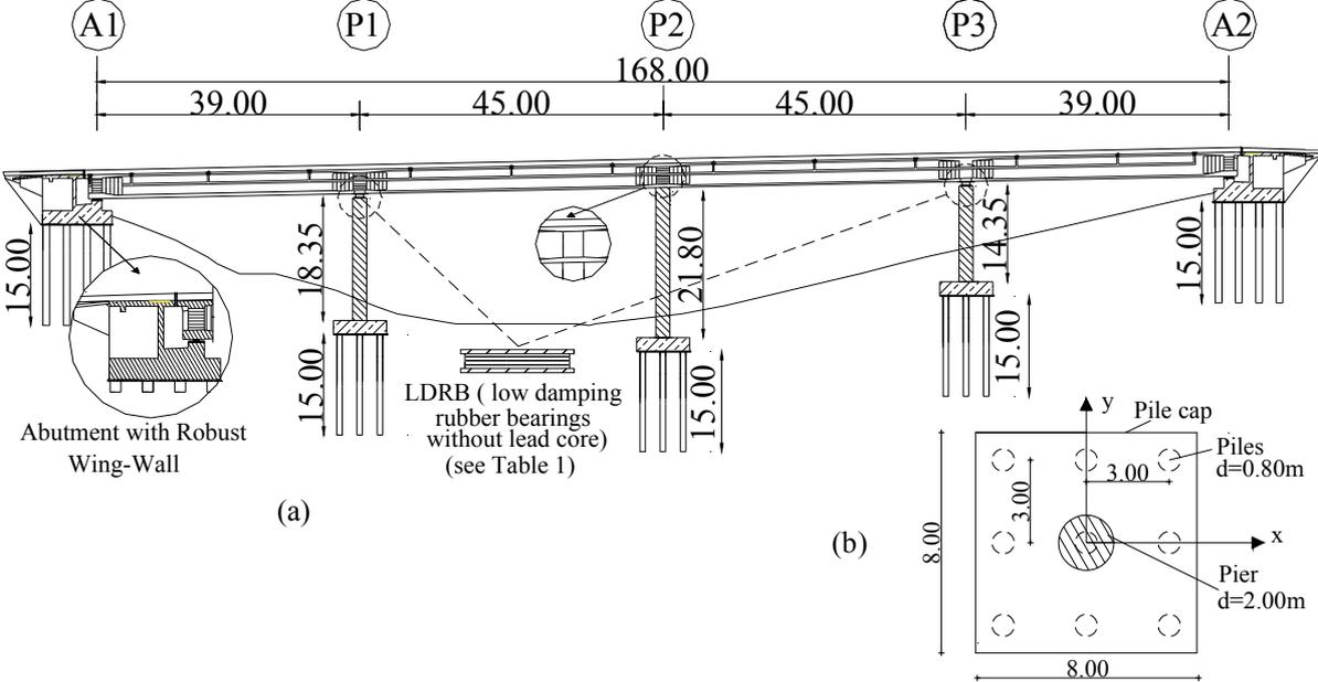
Figure 5. (a) Longitudinal section of the bridge BM<sub>2</sub>, (b) Plan view of the pier’s re-designed foundation.
