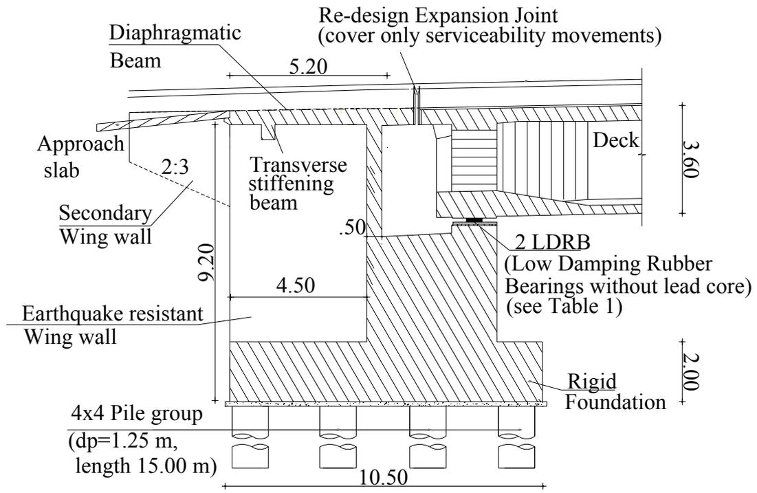
**Figure 3.** Longitudinal section of the proposed abutment with strong seismic participation
