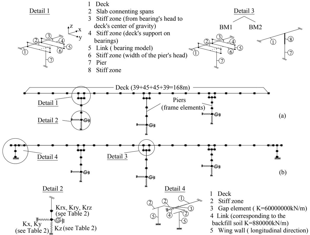
Figure 6. The model of: (a) Benchmark bridge, (b) Re-designed bridges
