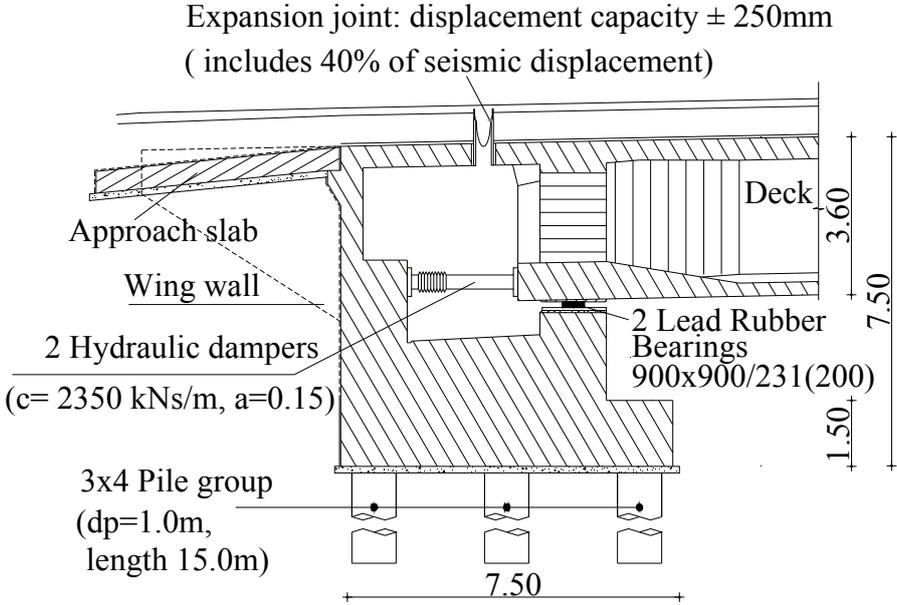
Figure 2. Longitudinal section of the as-built abutment
