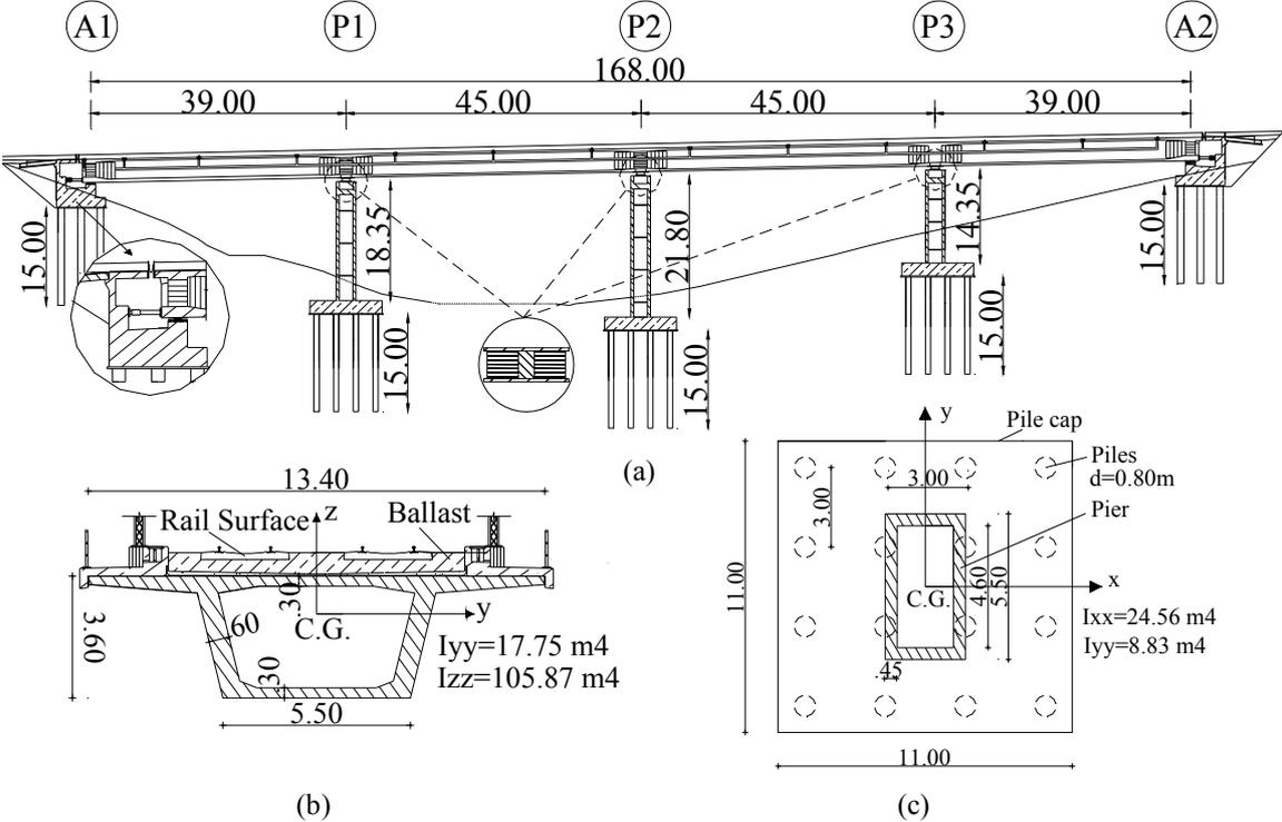
**Figure 1.** The benchmark bridge that belongs to OSE located at Polykastro, Greece, (a) Longitudinal section, (b) Cross section of the deck, (c) plan view of the pier’s foundation.
