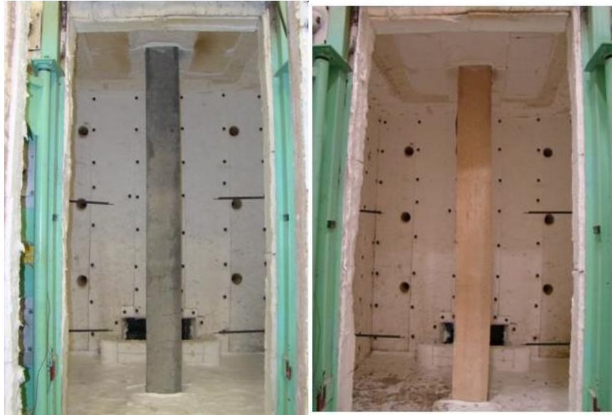
Figure 11. Column Specimen before, on the Left, and just after the Fire Test, on the Right.
