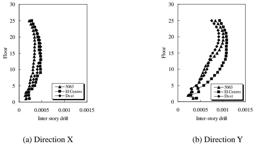
**Figure 4.4.** Analytical results of inter-story drift
