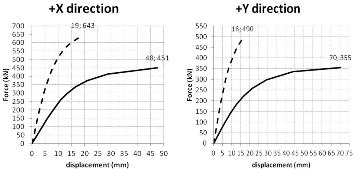
Figure 9. Capacity curves obtained with Acca Edilus. a) x-direction. b) y-direction
