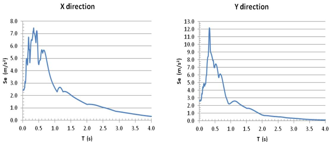
**Figure 4.** Response spectra of Kalamata earthquake, Greece 1986
