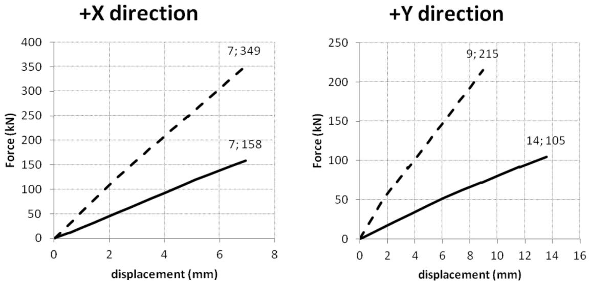
Figure 8. Capacity curves obtained with Aedes PC.E. a) x-direction. b) y-direction
