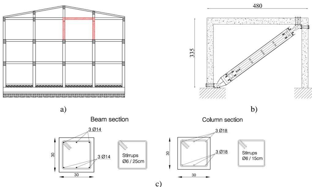
**Figure 7.** a) location of the isolated frame within the building b) main dimensions of the frame c) beam and column cross sections.
