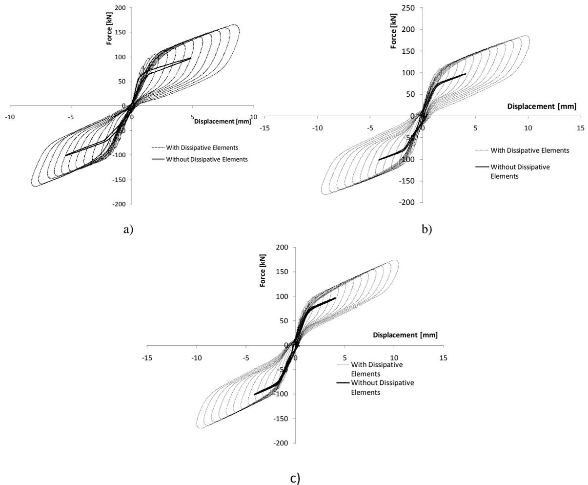
**Figure 13.** Force-displacement curve of the SSCD with Dissipative Elements, a) test 1, b) test 2 and c) test 3.
