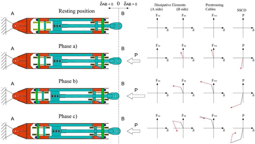
Figure 2 Main phases of the SSCD behavior under external compression force
