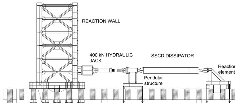
**Figure 10.** Test setup front view.
