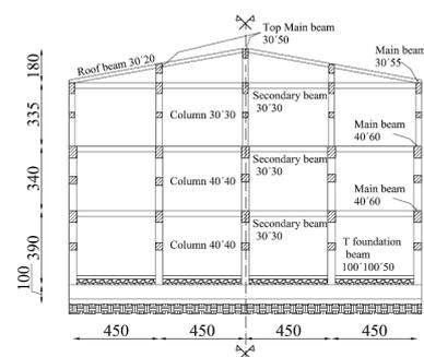
Figure 6. Case study: front view of the secondary external frames of the building.
