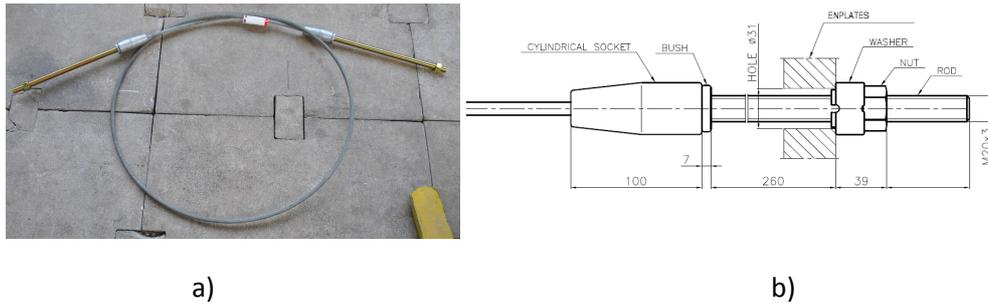
**Figure 9.** a) Prestressing Cables and b) cylindrical socket detail
