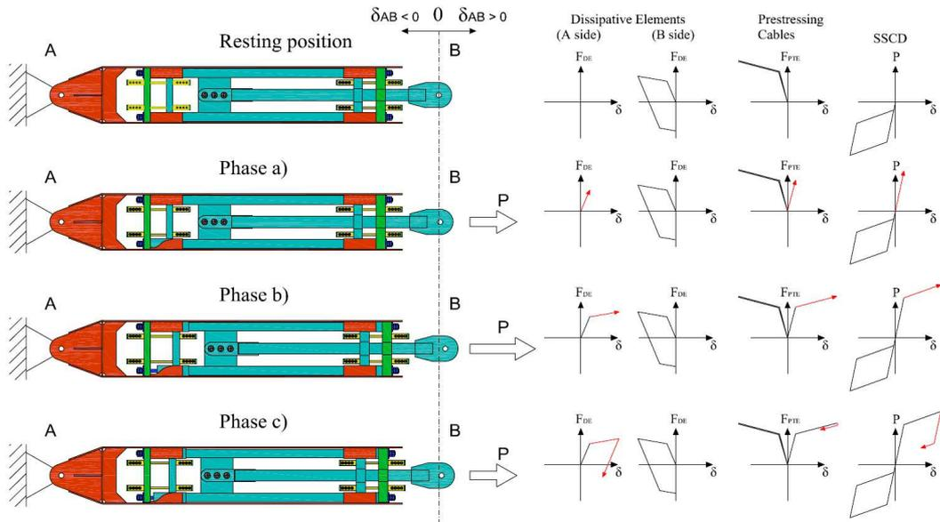
Figure 3. Main phases of the SSCD behavior under external tensile force after compression cycle.
