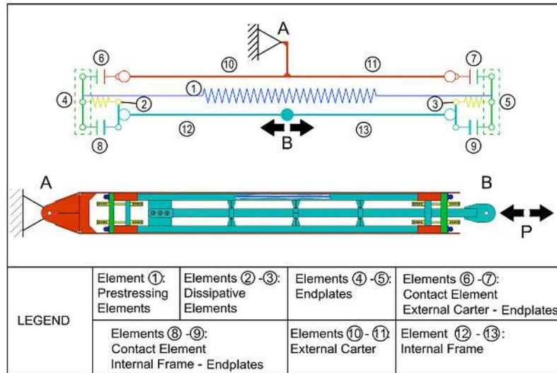
**Figure 8.** Simplified mechanical model of the SSCD
