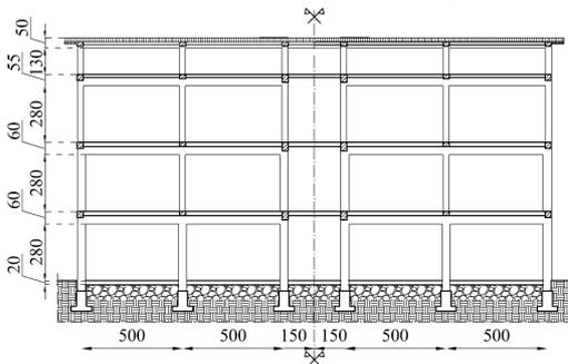
Figure 5. Case study: front view of the main frames in correspondence of the top of the roofing.
