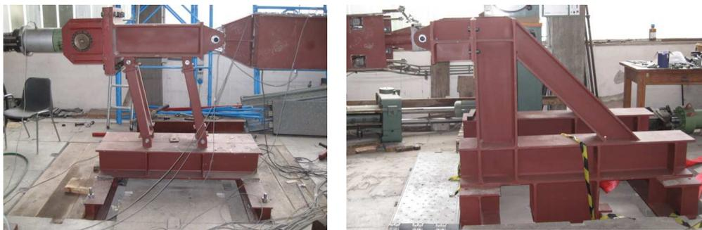
**Figure 11.** a) Pendular steel structure. b) Steel reaction element.
