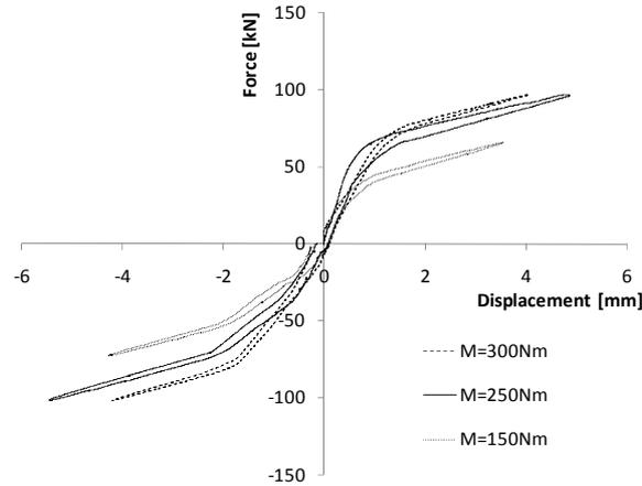
**Figure 12.** Force-displacement curve of the SSCD without the Dissipative Elements.
