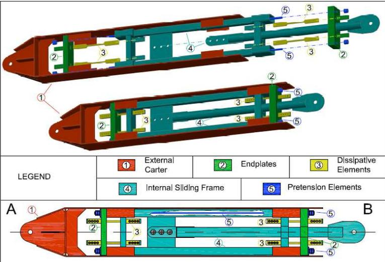
**Figure 1.** Main elements of the SSCD
