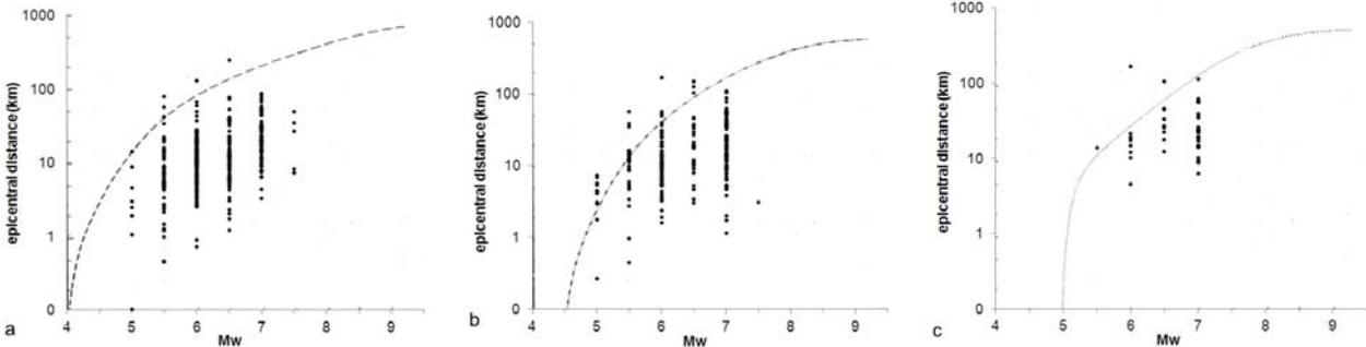
**Figure 7.** “Upper bound” curves representing the maximum distances at which earthquake-induced landslides can be expected (from Keefer, 1984) and data from the CEDIT catalogue referred to disrupted (a), coherent (b) and flow (c) landslides.
