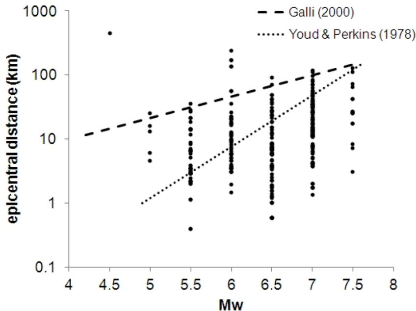
**Figure 8.** “Upper bound” curves representing the maximum distances at which liquefaction can be expected (by Youd & Perkins, 1978 and Galli, 2000) and liquefaction data from the CEDIT catalogue.
