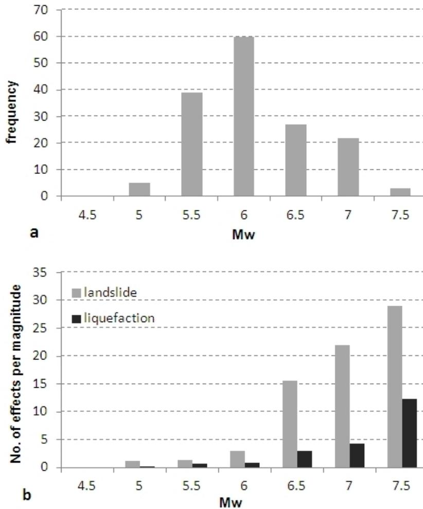
**Figure 5.** Frequency distribution of earthquakes that triggered ground failures (a) and the rate of ground failures per magnitude class (b).
