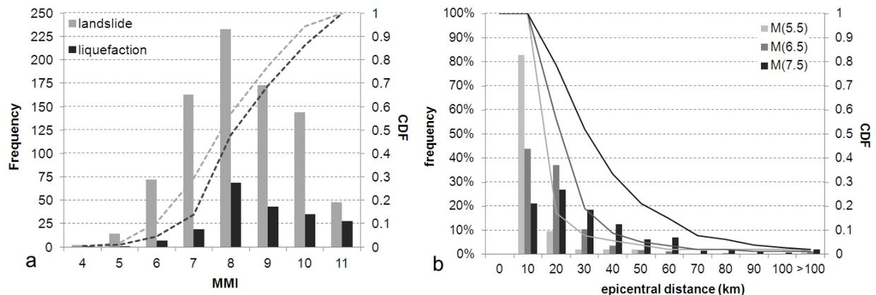
**Figure 9.** Probability of occurrence of earthquake-induced landslides and liquefaction as a function of MMI (a) and probability of occurrence of earthquake-induced landslides as a function of epicentral distance (b).
