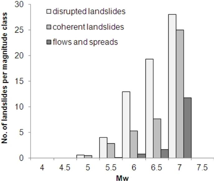
**Figure 6.** Number of landslides per magnitude class according to the Keefer’s (1984) seismic landslide categories.
