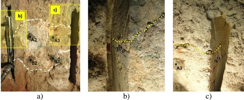
**Figure 7.** Shear failure: a) frontal cracks and details from the top crack inside the vertical cuts; b) left lateral crack and; c) right lateral crack (dimensions in cm).
