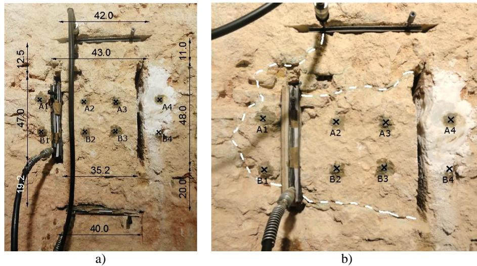
**Figure 9.** Shear Test 2: a) test setup with a vertical pressure of 0.60 MPa (dimensions in cm); b) frontal cracks on the masonry at the end of the test.
