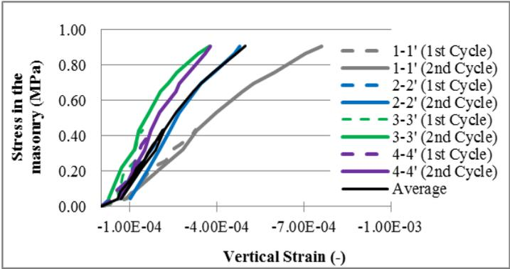
Figure 3. Relation between stress in the masonry and vertical strain.
