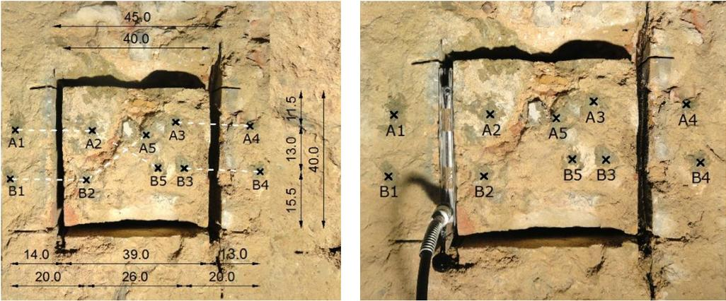
Figure 12. Shear flat-jack test setup and gage point's position (dimensions in cm).
