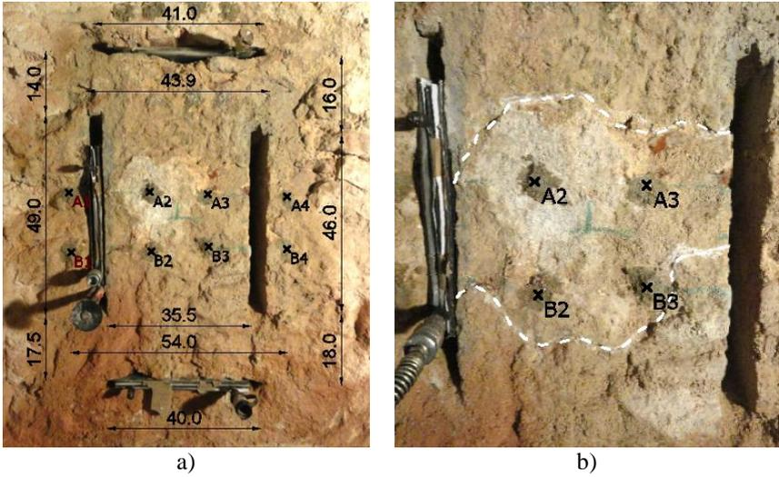
**Figure 5.** Shear Test 1: a) test setup with a vertical pressure of 0.40 MPa (dimensions in cm); b) frontal cracks on the masonry at the end of the test.
