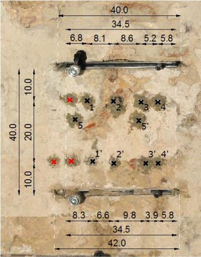
Figure 2. Double flat-jack test setup (dimensions in cm).
