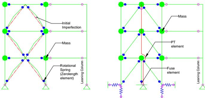
Figure 5. Proposed finite element models for original (3-story) building (a) IVBF, (b) single rocking
