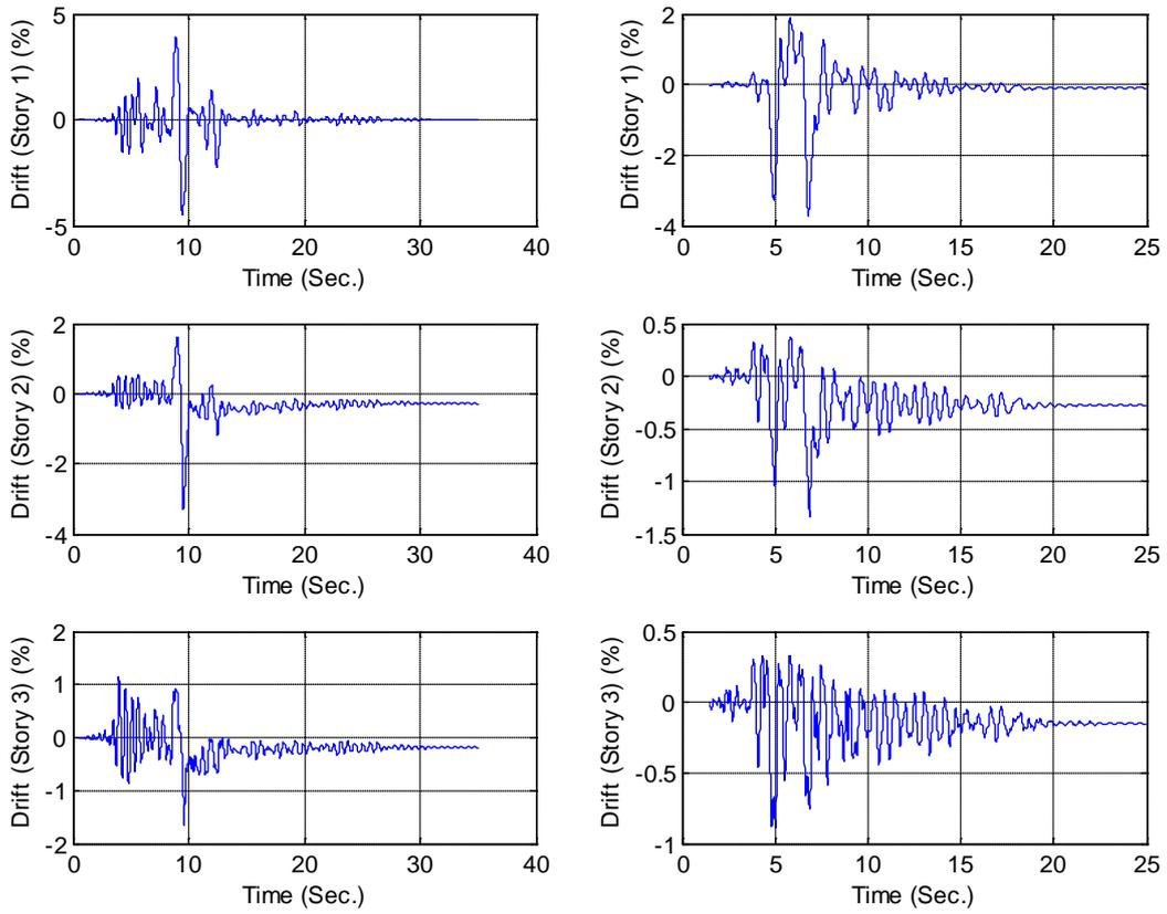
**Figure 8.** Story drift of IVBF subjected to MUL-279 (left) and LOS000 (right) earthquake records at MCE level
