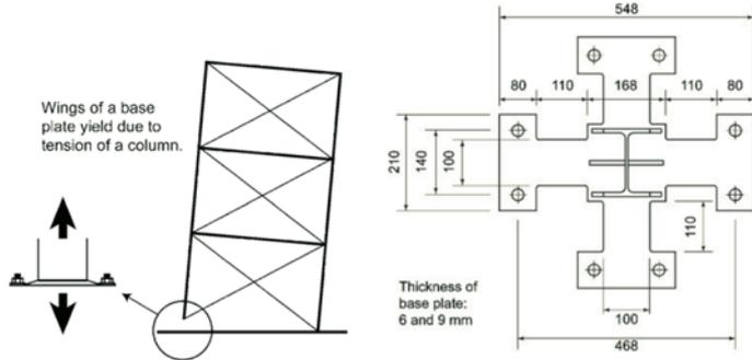
Figure 1. Base Plate Yielding (BPY) rocking system [6]: (a) configuration, (b) base plate detail
