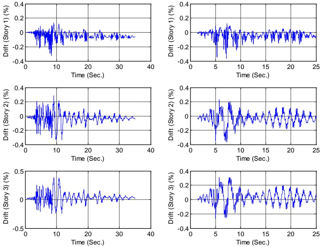
**Figure 9.** Story drift of SRS subjected to MUL-279 (left) and LOS000 (right) earthquake records at MCE level
