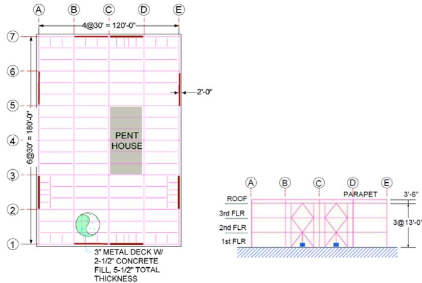
**Figure 3.** Prototype building [10] , [17] (a) typical plan, (b) elevation
