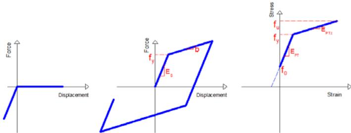
Figure 6. Material models: (a) elastic no tension, (b) calibrated steel fuse, (c) PT component
