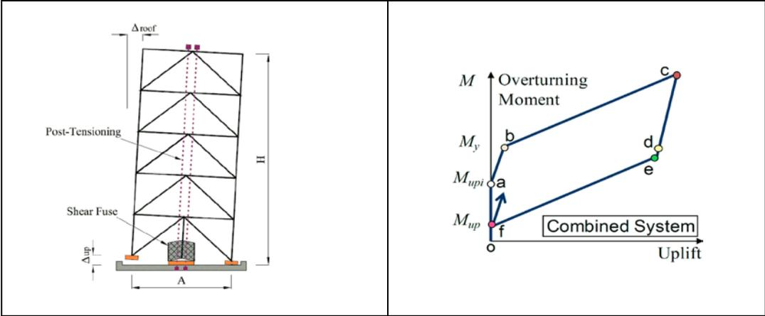
Figure 2. Single rocking system [10]: (a) configuration, (b) backbone curve
