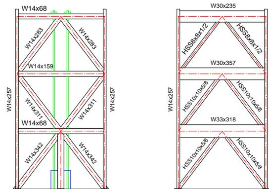
**Figure 4.** Structural system specification for original (3-story) building (a) single rocking [10], (b) IVBF
