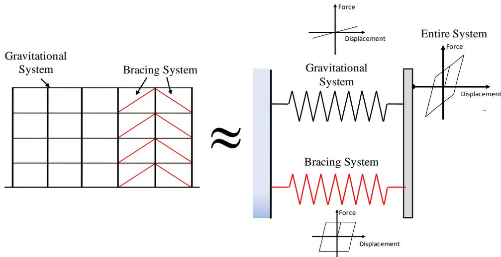
**Figure 1.** Behavior of a damage-tolerant building conceived according to the UAM approach
