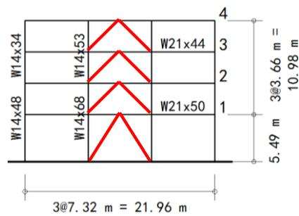
Figure 4. Configuration of bracing system for the four and eight-story frames
