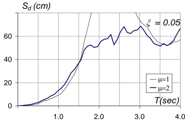
Figure 7. Design spectra for the twenty-four-story building
