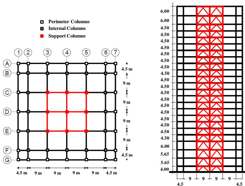
Figure 5. Geometry and structural layout of twenty four-story building
