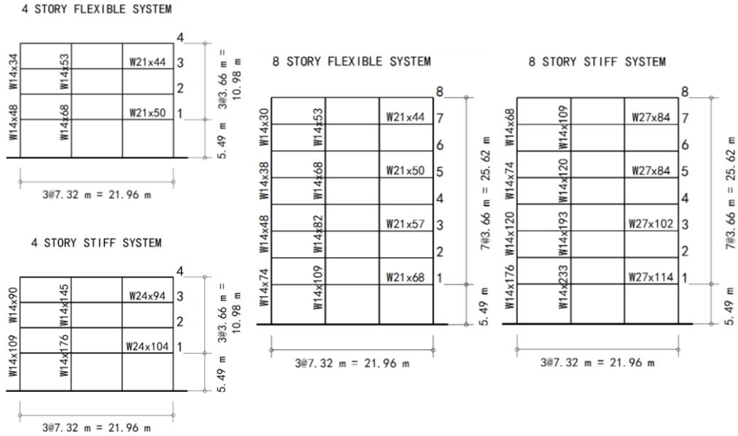
Figure 3. Steel moment-resisting frames under consideration (Santa Ana and Miranda 2000)
