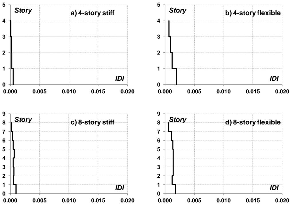
**Figure 9.** Permanent interstory drift index demands for the four and eight-story frames
