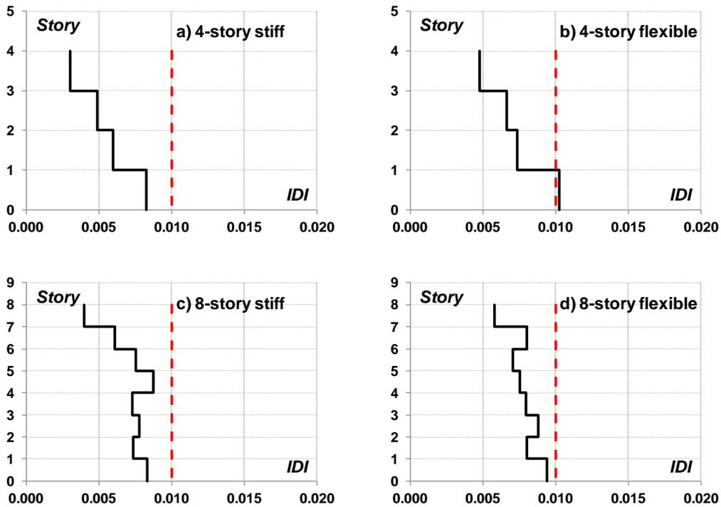
**Figure 8.** Maximum interstory drift index demands for the four and eight-story frames
