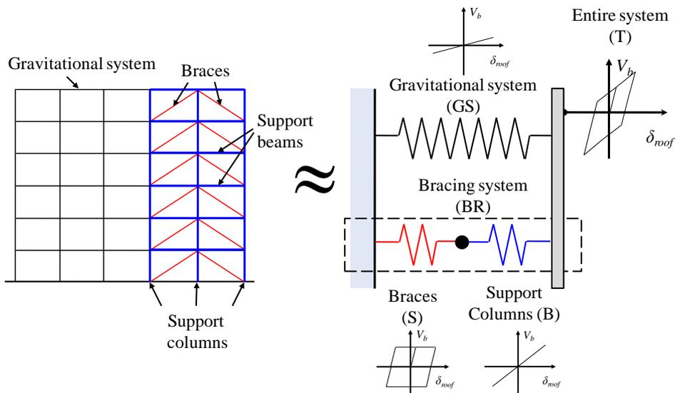
**Figure 2.** Modeling assumptions for tall buildings stiffened with a bracing system
