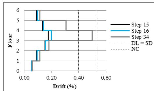
**Figure 11.** Structure's interstorey drifts and compliance limits.
