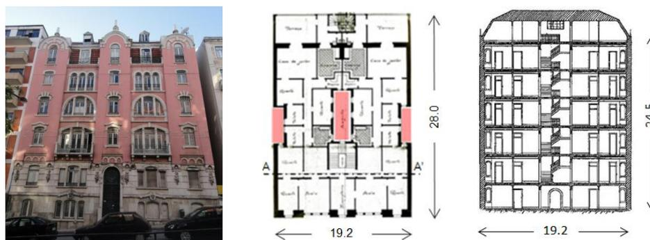
**Figure 1.** Façade wall of the building, plan drawing of a current floor and cut AA' (dimensions in meters).
