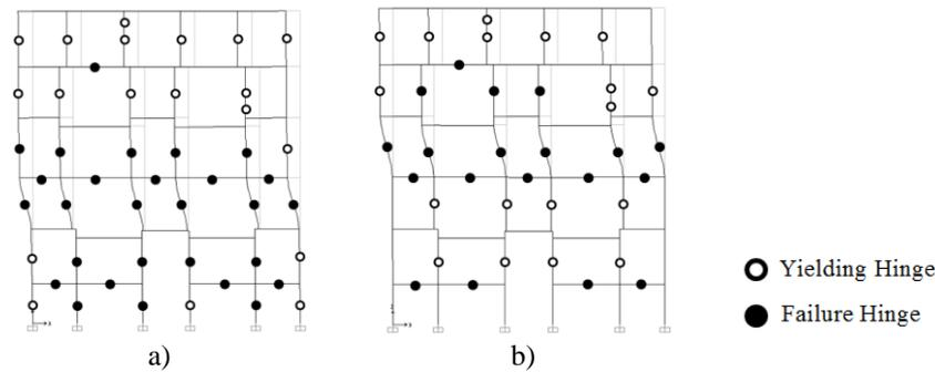
**Figure 7.** Plastic hinges distribution at the final stage of Case 3: a) Uniform Load; b) Modal Load.
