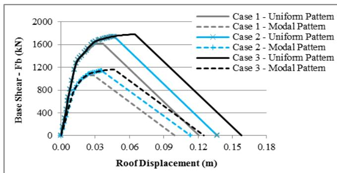
**Figure 6.** Façade wall capacity curves.**Table 2.** Capacity curve's ultimate results.
