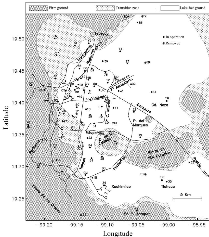
Figure 3. Accelerometer network of the valley of Mexico (Mexican Strong Earthquakes Ddata Base, 1999)
