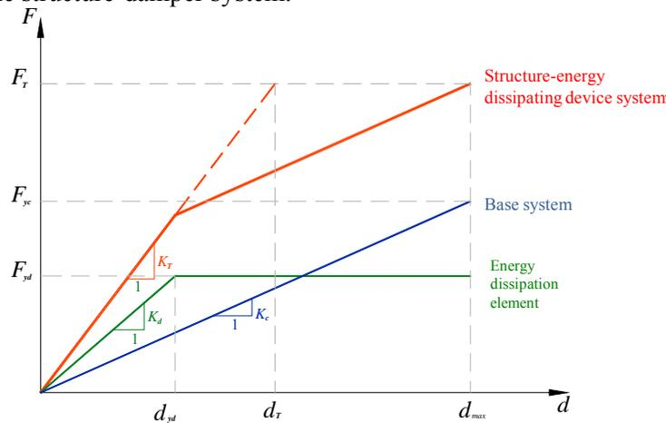
**Figure2.** Force-displacement curves of the parts constituting the structure-damper system
