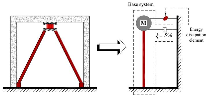
**Figure1.** Model of the structure-energy dissipating device system
