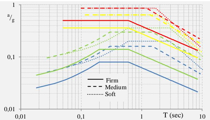
Figure 2. Spectrum designs according with CFE (1993).
