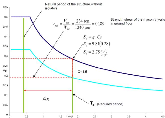
**Figure 7.** Spectral design, traditional structure period and the proposed isolated building period
