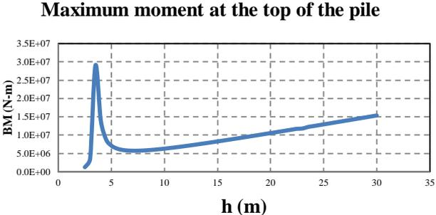
**Figure 1.** Variation of the bending moment at the base of a pier with pier height for  $v=100$  m/s,  $L=10$  m,  $r=0.5$  m and  $M=50000$  kg
