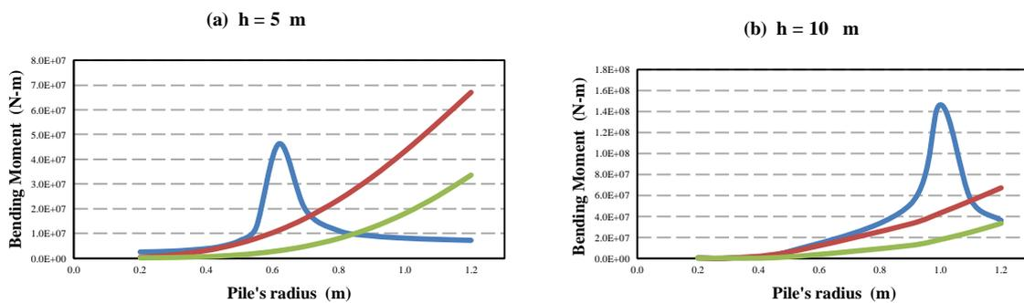
**Figure 3.** Variation of the bending moment with pile radius for  $M = 50000$  kg, continuous, dash-dot and dashed lines are respectively for  $MB$ ,  $BM_b$  and  $BM$ .
