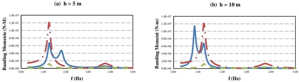
**Figure 4.** Variation of the bending moment with the normalized frequency for  $\nu=100$  m/s,  $L=20$  m,  $r=0.5$  m and  $h=5$  m  $M=50000$  kg, continuous, dash-dot and dashed lines are respectively for  $MB$ ,  $BM_b$  and  $BM_t$ .
