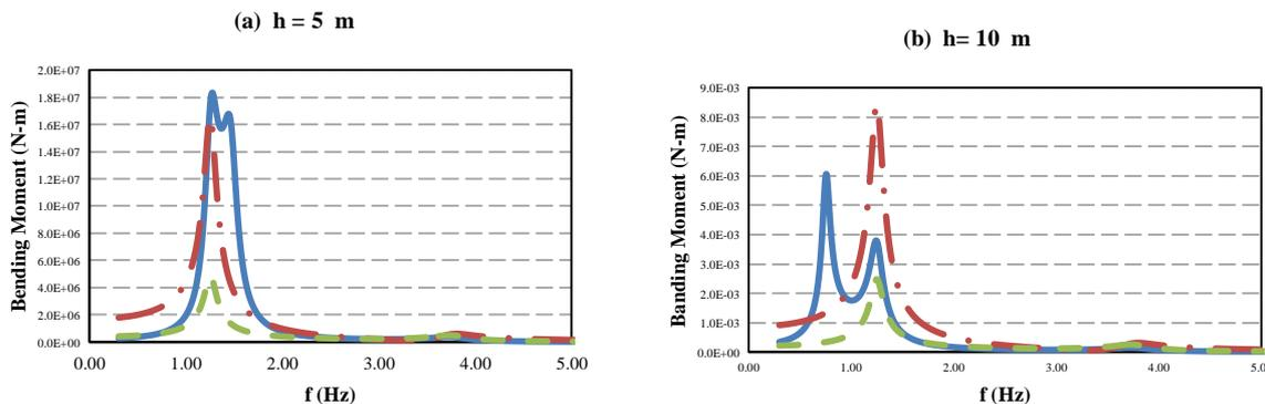
**Figure 5.** Variation of the bending moment with the normalized frequency for  $\nu=50$  m/s,  $L=10$  m,  $r=0.5$  m and  $M=50000$  kg, continuous, dash-dot and dashed lines are respectively for  $MB$ ,  $BM_b$  and  $BM_t$ .
