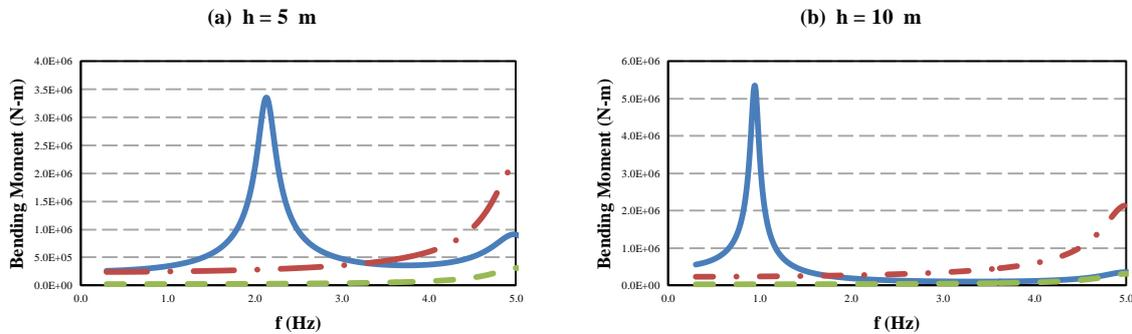
**Figure 6.** Variation of the bending moment with the normalized frequency for  $v=200$  m/s,  $L=10$  m,  $r=0.5$  m and  $h=5$  m  $M=50000$  kg, continuous, dash-dot and dashed lines are respectively for  $MB$ ,  $BM_b$  and  $BM_t$ .
