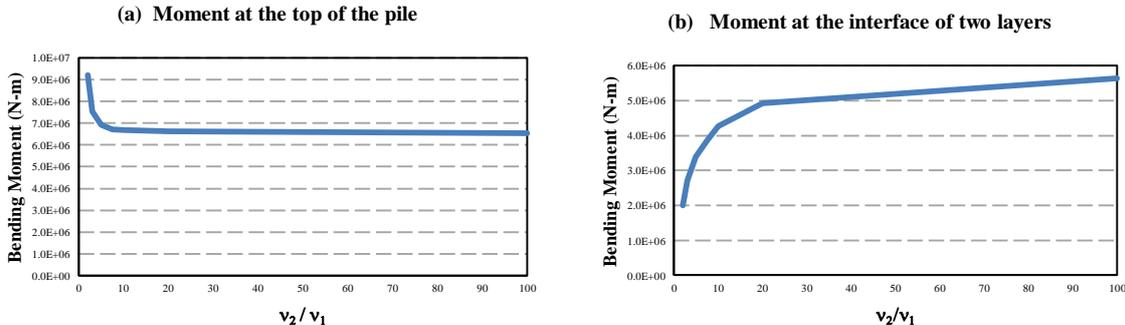
Figure 7. Variation of the bending moment at the top of the pile vs.  $v_2 / v_1$
