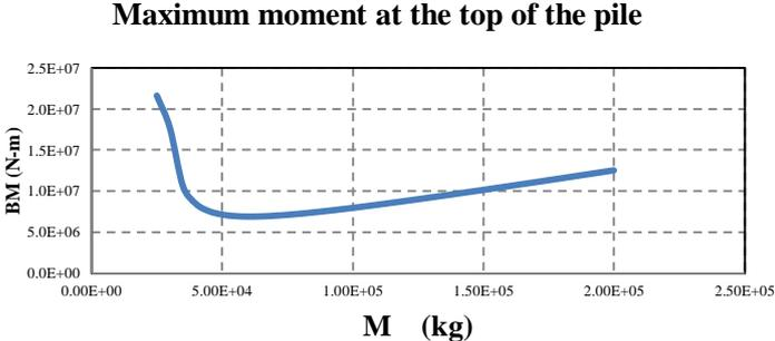
**Figure 2.** Variation of the bending moment at the base of a pier with top mass for  $v=100$  m/s,  $L=10$  m,  $r=0.5$  m and  $h=5$  m
