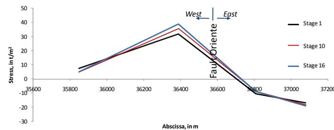
**Figure 10.** Resultant stresses in the zone of Oriente fault
