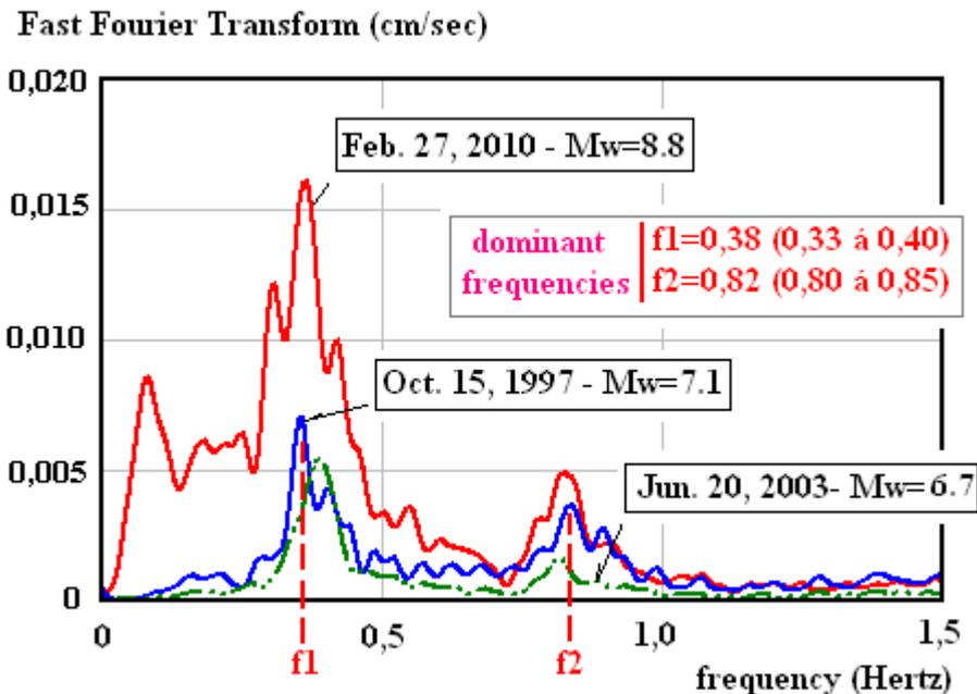
Figure 5.3 – Fast Fourier Transform of Three of the Chilean Accelerograms Listed in Table 5.1
