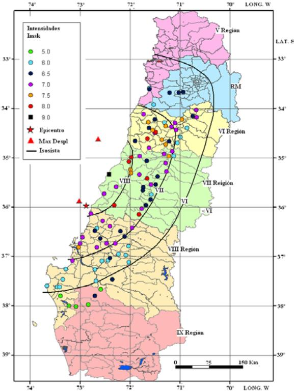
**Figure 2.1** – 2010 Great Chilean Earthquake- Seismic Intensities. (Astroza M. et al, 2010)
