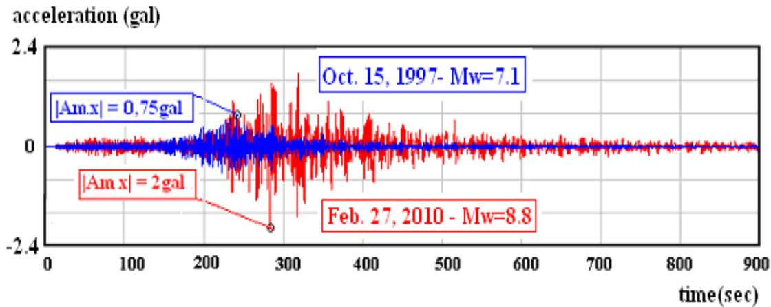
**Figure 5.2-** N-S Components of La Plata Accelerograms of Feb.27, 2010 Mw=8.8 and Oct. 15, 1997 Mw=7.1
