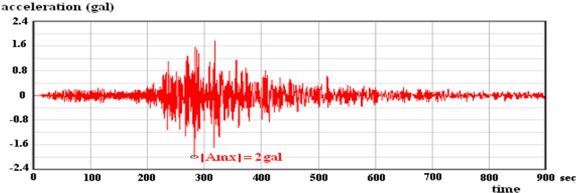
Figure 3.1- N-S Component of La Plata Acelerogram Recorded During 2010 Great Chilean Earthquake
