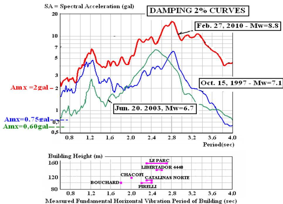
Figure 6.1 – Damping 2% Acceleration Response Curves and Building Horizontal Vibration Period
