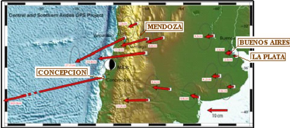
Figure 2.2- 2010 Great Chilean Earthquake – Displacement of Earth Crust by GPS (Barrientos S.,2010)
