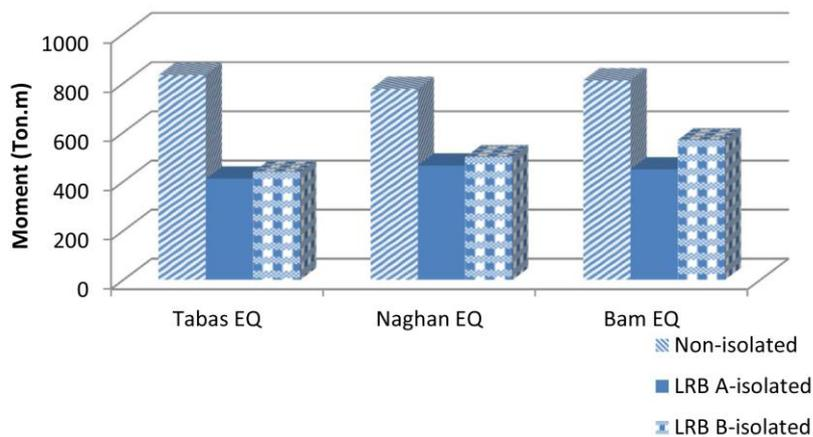
**Figure 5.4.** Maximum moment in one of the piers of the bridge in various bearing condition and under three different strong earthquake motions
