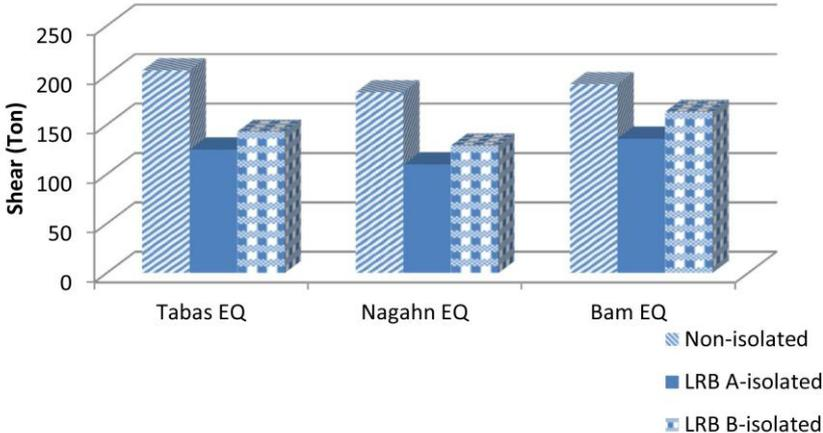
**Figure 5.2.** Maximum longitudinal shear in one of the piers of the bridge in various bearing condition and under three different strong earthquake motions
