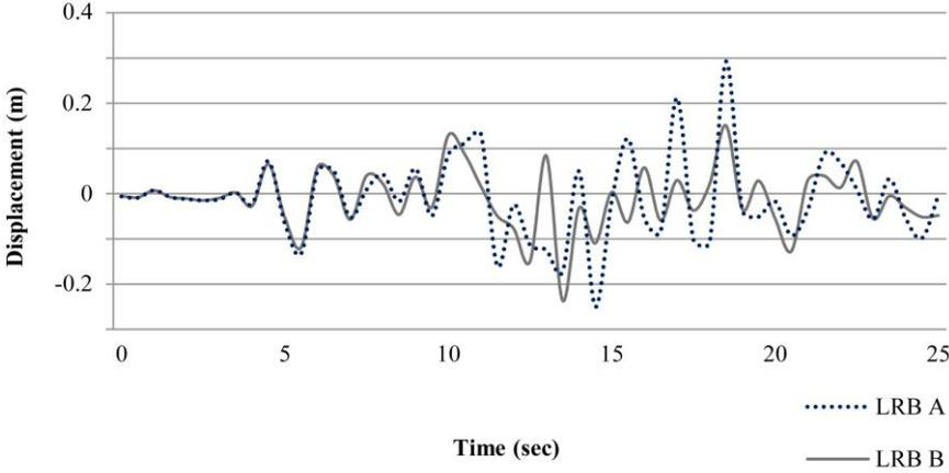
**Figure 5.1.** Time variation of longitudinal bearing displacement of the bridge isolated by LRB system under Tabas earthquake motion
