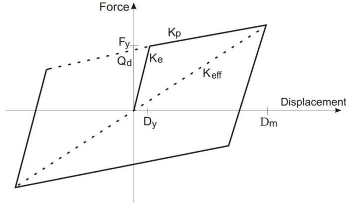
**Figure 4.1.** Bilinear force-displacement behaviour of LRB
