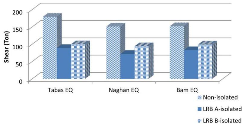
**Figure 5.3.** Maximum longitudinal shear in abutments of the bridge in various bearing condition and under three different strong earthquake motions
