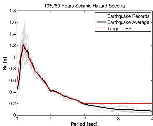
**Figure 2:** Ground motion records scaled to the target UHS
