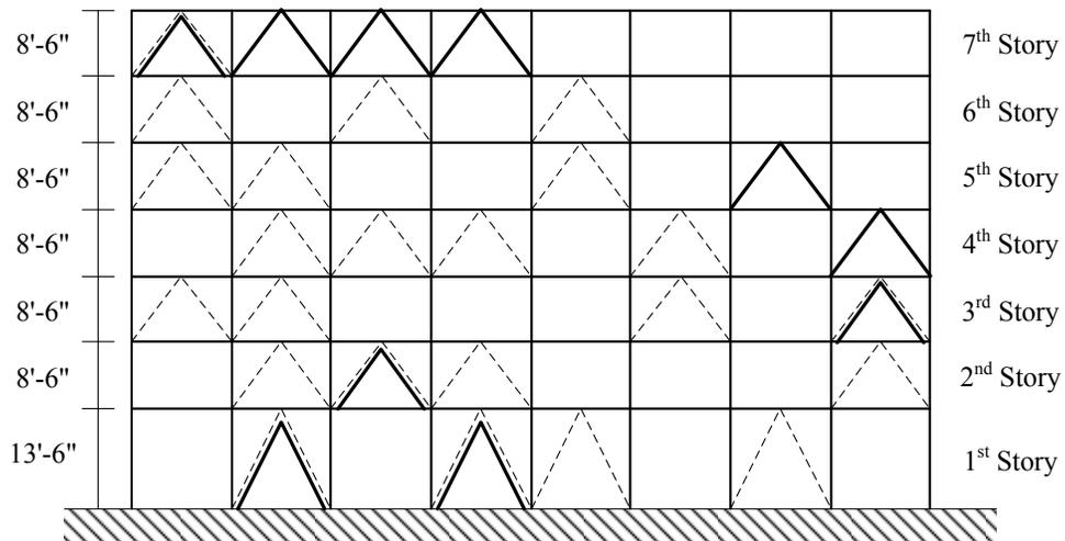
**Figure 4:** Van Nuys Hotel schematic with Sequential Search (Solid Lines) and Genetic Algorithm (Dashed Lines) optimized retrofit schemes
