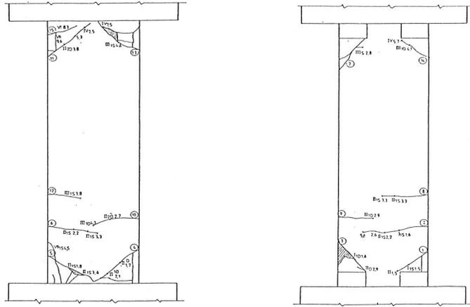
Figure 9. Model PI 1. Cracks pattern
