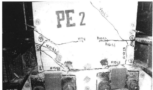
Figure 15. Detail after failure of model PE 2
