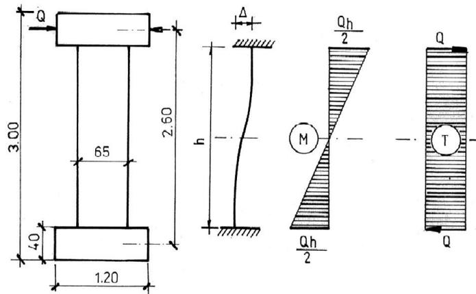
Figure 3. Experimental element
