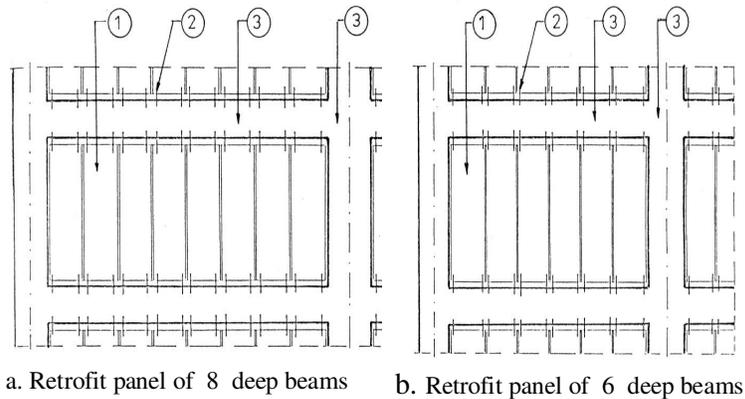
Figure 2. Retrofit precast panels
