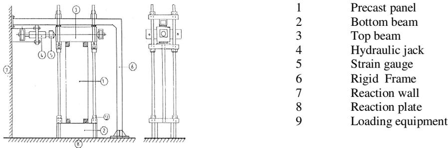
Figure 4. Test set-up
