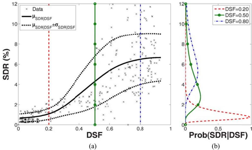
**Figure 3.3.** (a) Scatter plot of DSF versus maximum SDR and the conditional mean and standard deviation; (b) Conditional probability density function of SDR given DSF for the four-story steel SMRF
