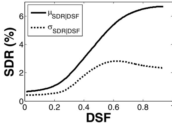
**Figure 3.4.** Conditional mean and standard deviation of SDR given DSF for the four-story steel SMRF
