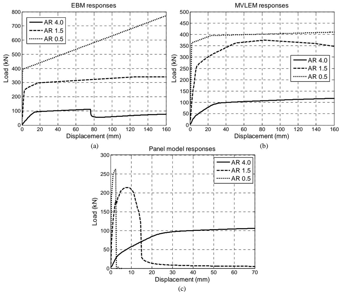
**Figure 5.2.** Load-displacement response for different aspect ratios
