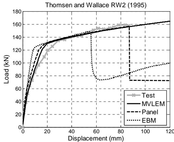
**Figure 4.1.** RW2: Load-displacement response
