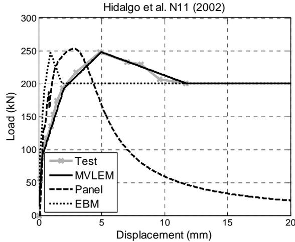
Figure 4.3. N11: Load-displacement response
