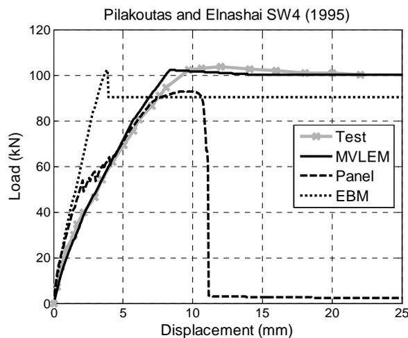
Figure 4.2. SW4: Load-displacement response
