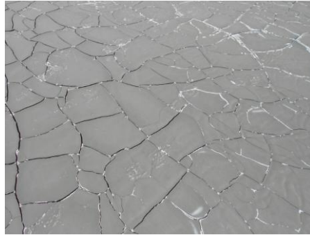
Figure 1. Typical desiccation crack pattern observed in a TTD in Chile
