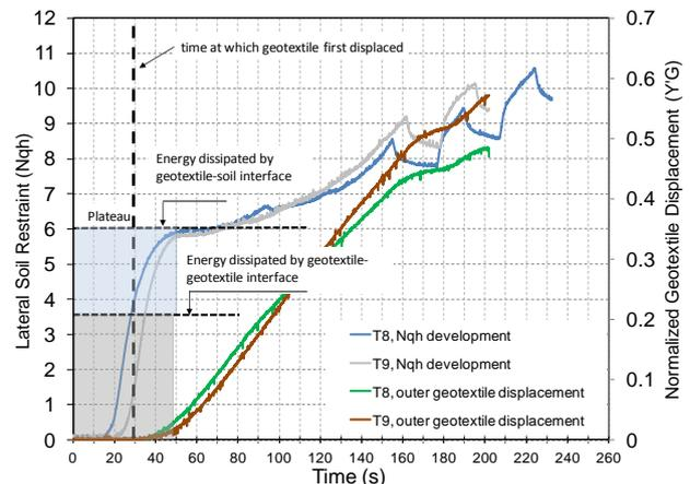
**Figure 4.6.** Evolution of lateral soil restraint and geotextile displacement for T8 and T9.
