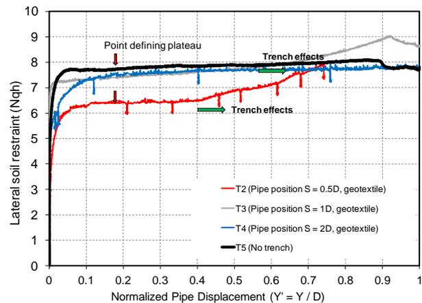
**Figure 4.2.** Effect of trench wall-pipe distance ( $S$ ) on levels of soil restraints.
