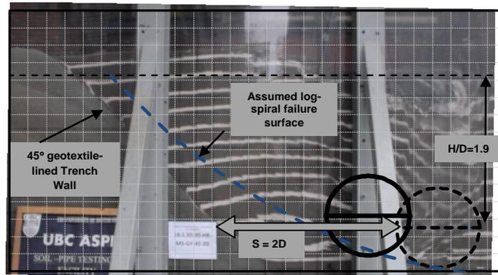
**Figure 4.3** Log-spiral failure surface developed for trench wall-pipe distance  $S = 2D$  (grid  $0.1 \times 0.1$  m).
