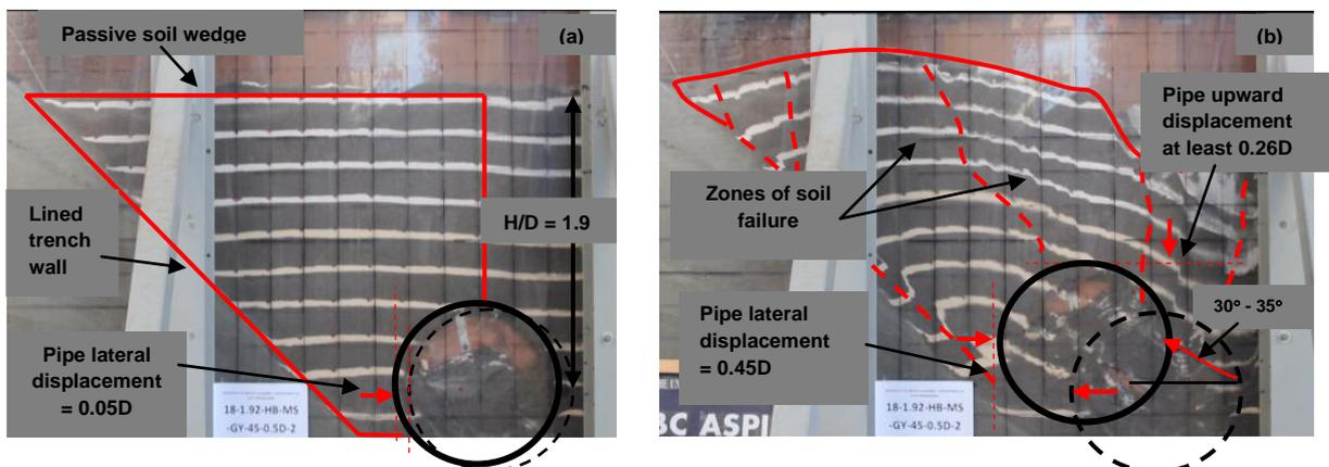
**Figure 4.4** Observed soil deformations for tests with moist sand backfill: (a) after  $Y'=0.05D$ , and (b) after  $Y'=0.45D$ . Note that grid on plexiglass is  $0.1 \times 0.1$  m.
