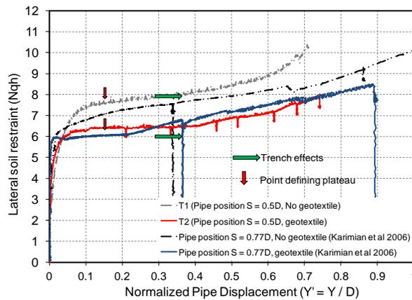
**Figure 4.1.** Lateral soil restraints in sloped trench walls with moist sand backfill.
