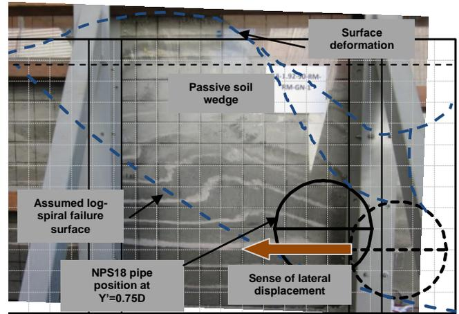
**Figure 4.8.** Log-spiral failure surface developed during Tests T10 and T11.
