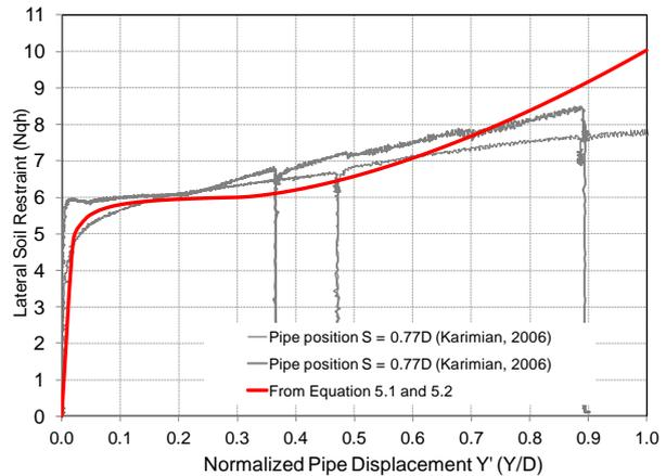
**Figure 5.3.** Soil restraint relationship from Equation 5.1 and 5.2 vs. data from Karimian et al (2006)
