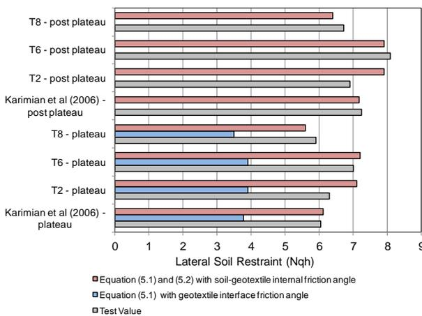
**Figure 5.2.** Comparison between restraints from tests and restraints from Equation 5.1 and 5.2. Post-plateau calculated at  $Y' = 0.5D$ .
