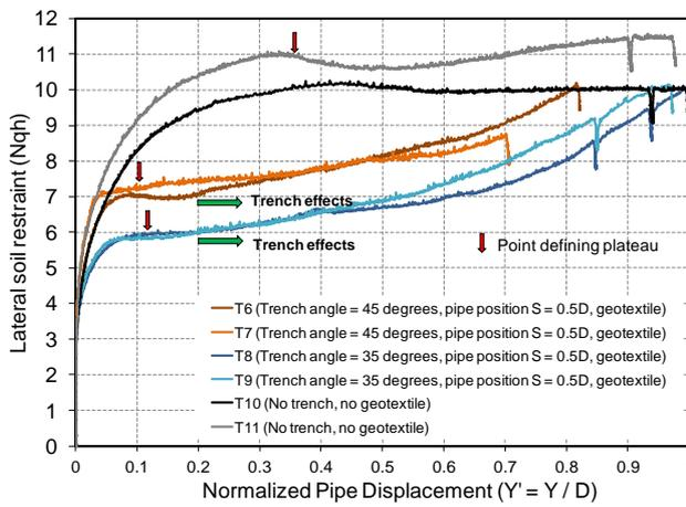
**Figure 4.7.** Lateral soil restraints in sloped trench walls with sand and gravel backfill.
