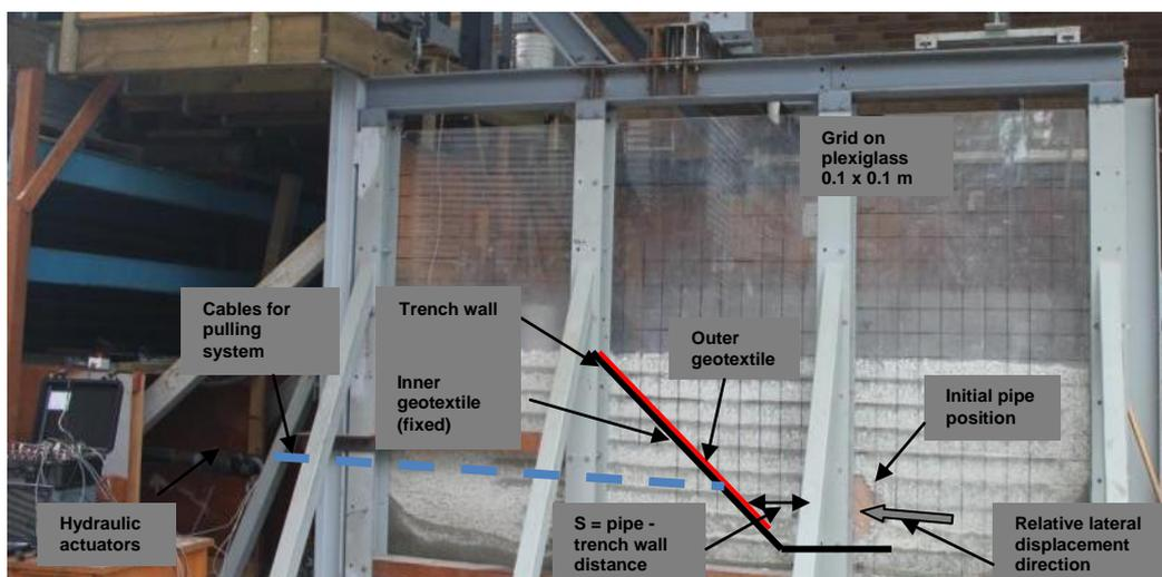
**Figure 2.1.** Perspective view of the testing chamber and general arrangements for tests.
