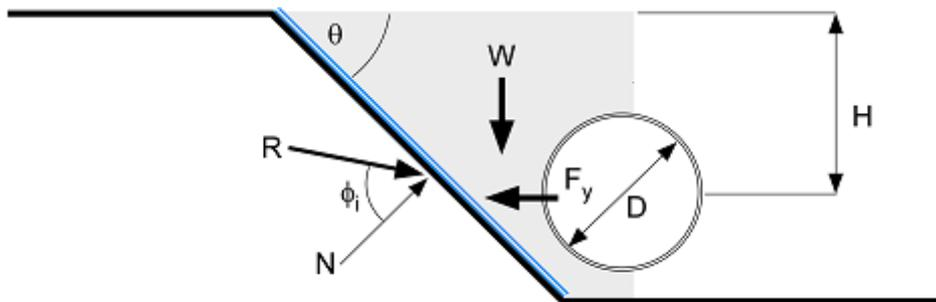
**Figure 5.1** Sliding block mechanism for quantifying  $F_y$  for pipeline systems with geotextile-lined trench walls.  $\phi_i$  is the geotextile-soil interface friction angle.
