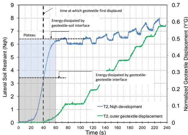
**Figure 4.5.** Evolution of lateral soil restraint and geotextile displacement as a function of time for T2.
