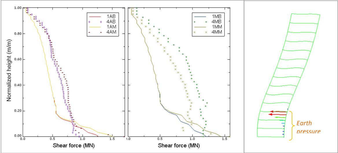
**Figure 10.** (Left) Maximum shear force envelope along the columns. (Right) Lateral earth pressure distribution at time of maximum shear.
