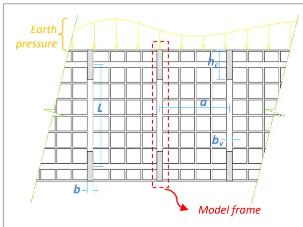
**Figure 2.** Typical floor plan of the analyzed structures.
