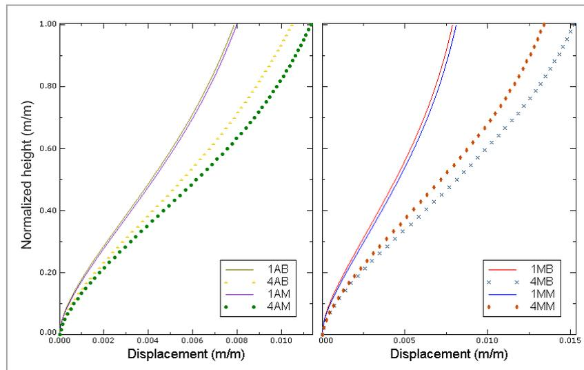
**Figure 9.** Maximum drift envelope along the columns.
