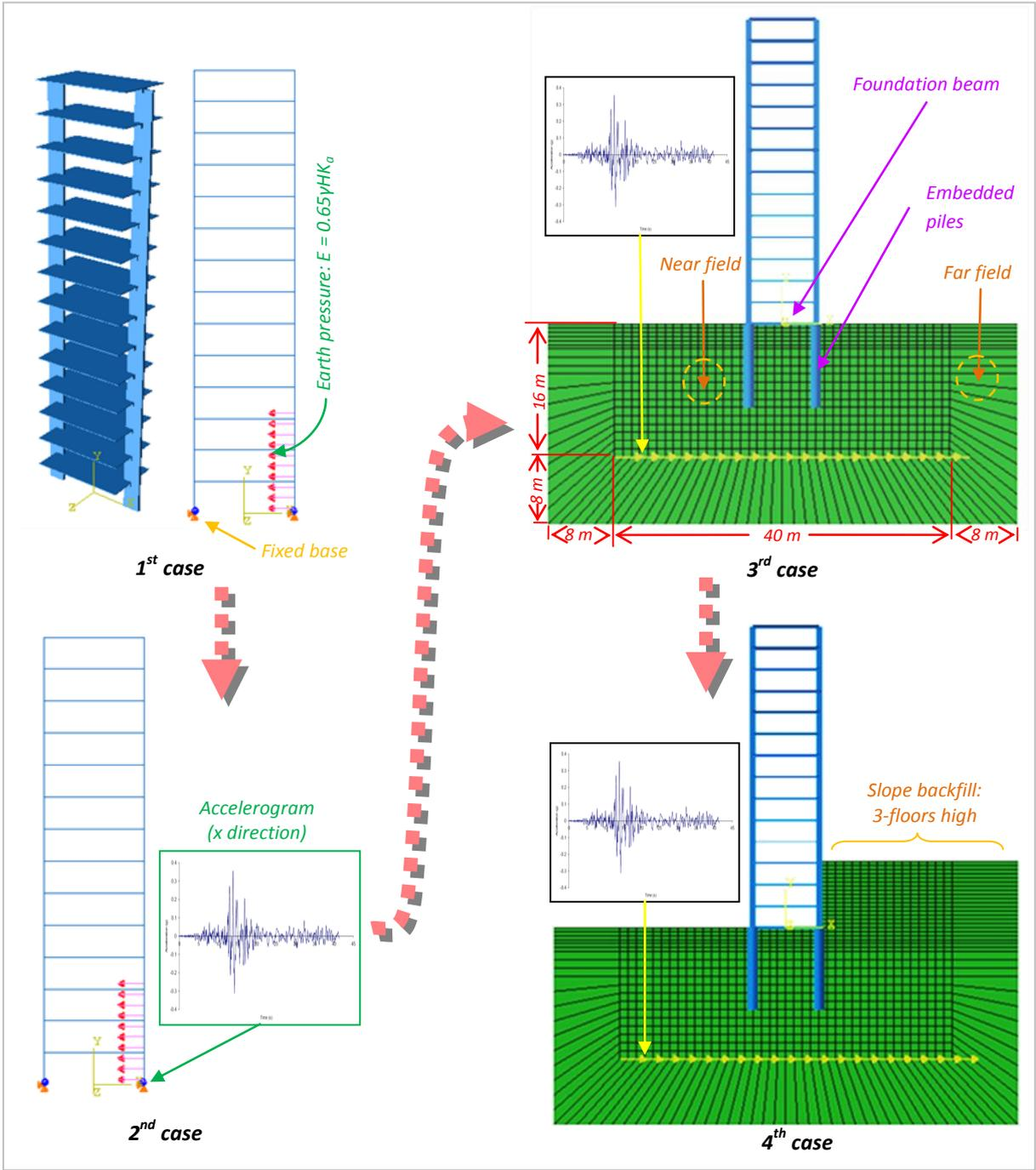
Figure 5. Sequence of finite elements models implemented.
