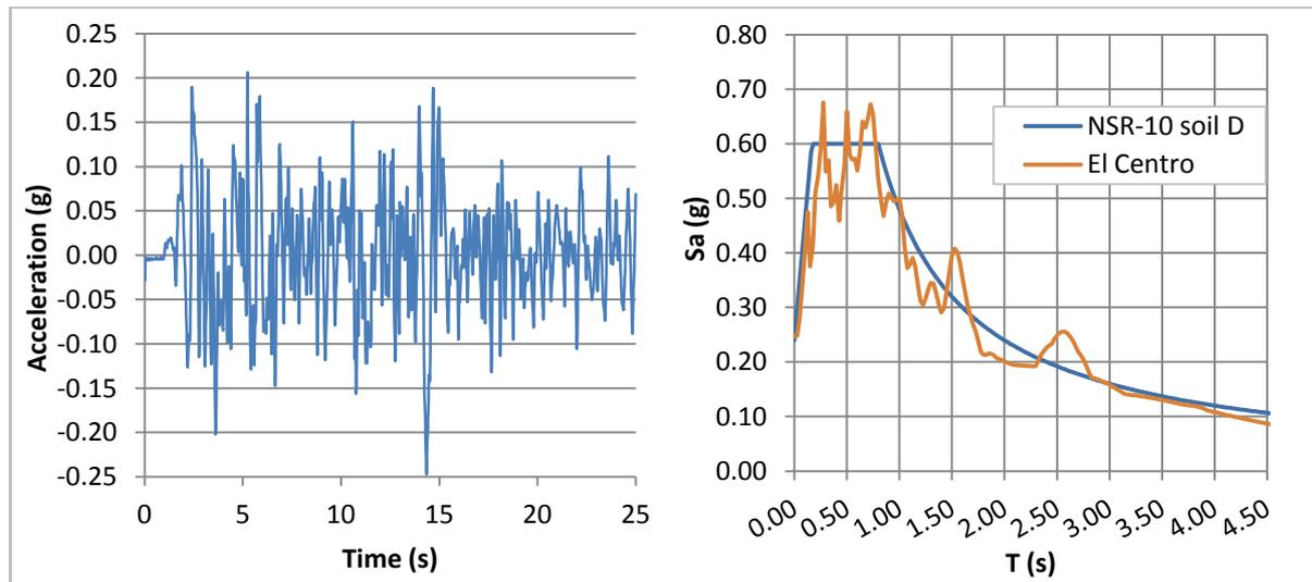
**Figure 6.** Seismic inputs used: (Left) El Centro EW accelerogram. (Right) Acceleration spectrum according to NSR-10 and compared to that of El Centro EW.
