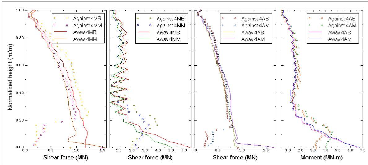
**Figure 8.** Maximum shear forces and overturning moments for both directions of the structure's movement.
