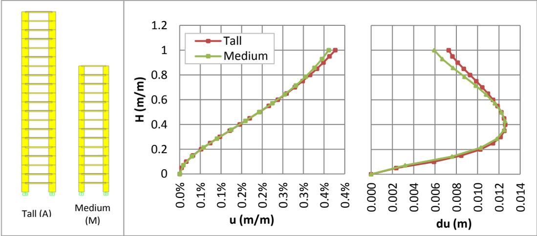
**Figure 3.** (Left) Two-dimensional frames modeled for buildings *A* and *M*. (Right) Displacement,  $u$ , and story drift,  $du$ , for both frames resulting from a modal response spectrum analysis.
