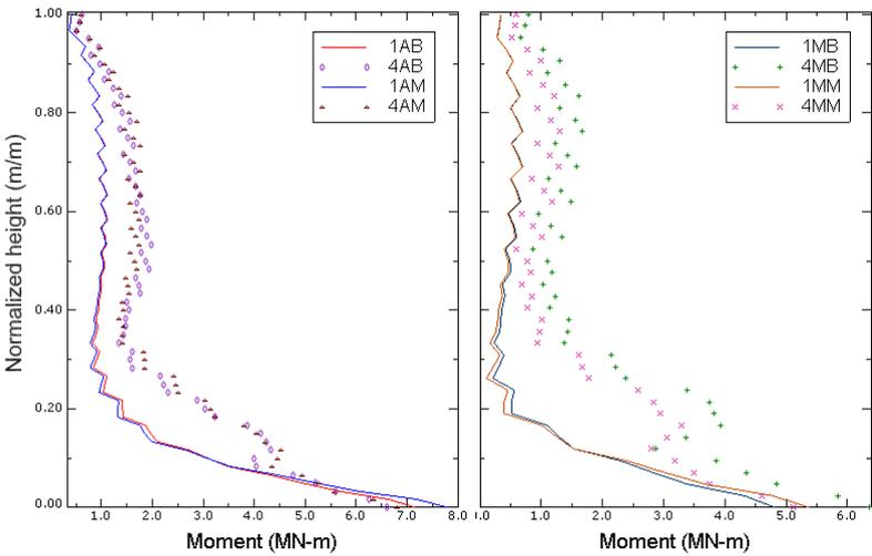
**Figure 11.** Maximum overturning moment envelope along the columns.
