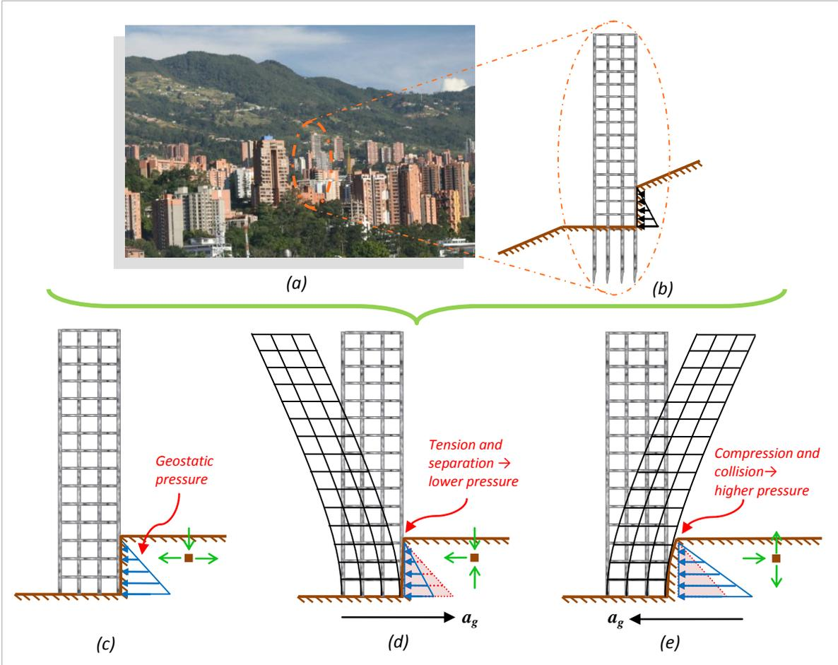
**Figure 1.** Outline of the situation under study: (a) Buildings on sloping ground in Medellín, Colombia; (b) Vertical plane showing the asymmetric lateral earth pressure against the building; (c) static conditions; (d) movement of the structure in the direction of soil pressure and (e) against the direction of soil pressure.
