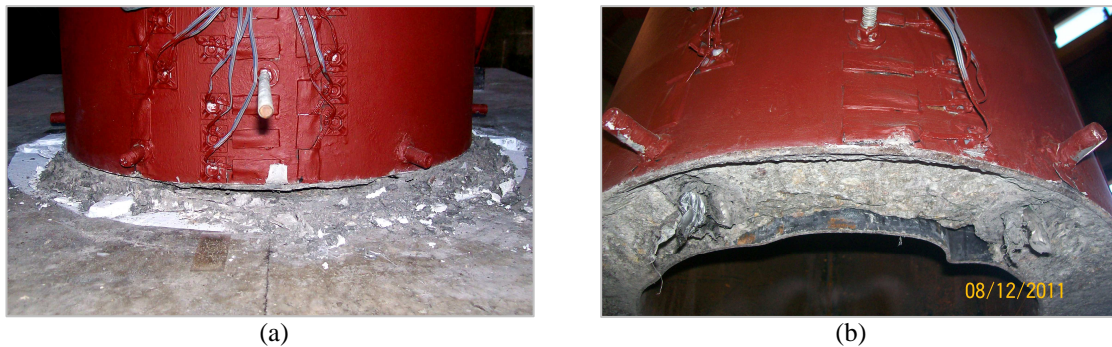
Figure 9. Unit 1B after testing: (a) crushed mortar bed; (b) permanent deformations of concrete and steel shells.
