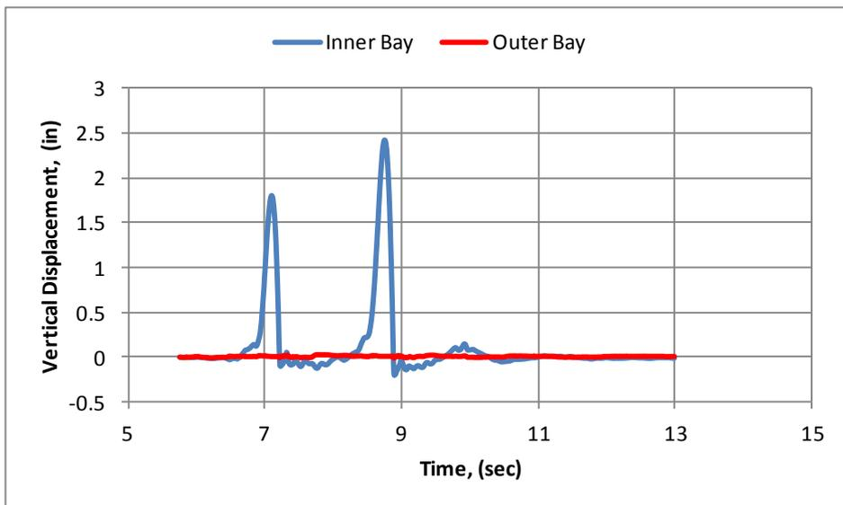
**Figure 4.6:** Vertical Uplift at North Abutment at 350% of the Design Earthquake
