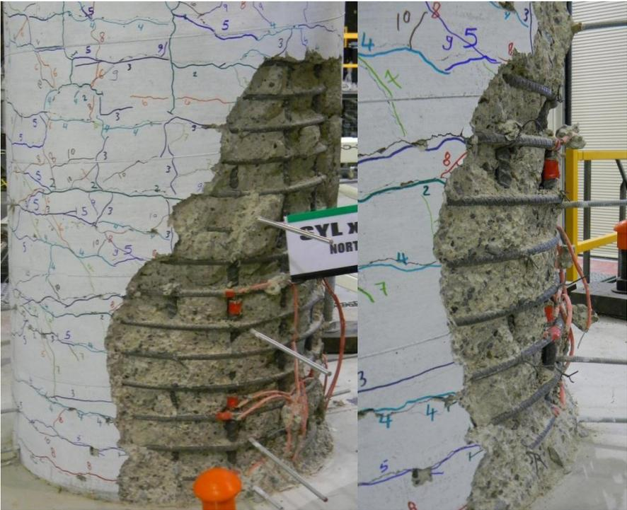
**Figure 4.2: South Bent @ 350% of Design Earthquake**
