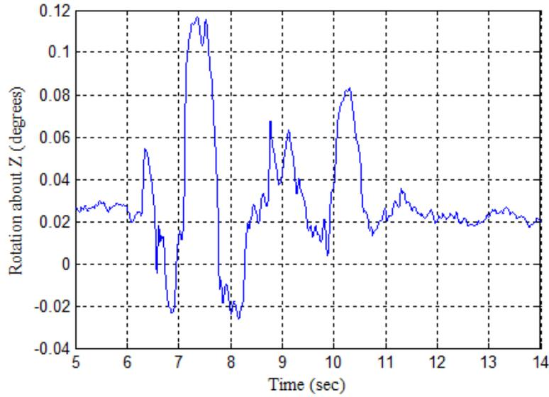
**Figure 4.8:** South Bent Rotation vs. Time @ 100% Design Earthquake
