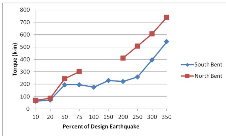
**Figure 4.9:** Column Torque
