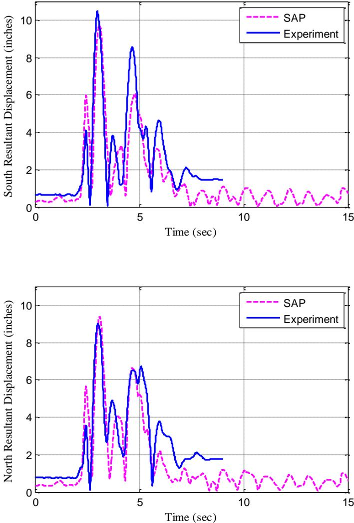
**Figure 5.1:** Resultant Displacement Comparison @ 350% Design Earthquake
