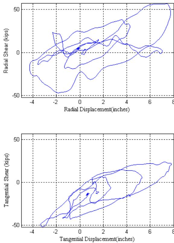
**Figure 4.4:** South Bent Shear vs. Displacement @ 350% Design Earthquake
