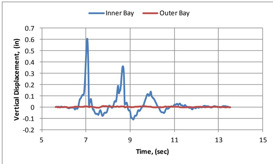
**Figure 4.5:** Vertical Uplift at North Abutment at 300% of the Design Earthquake
