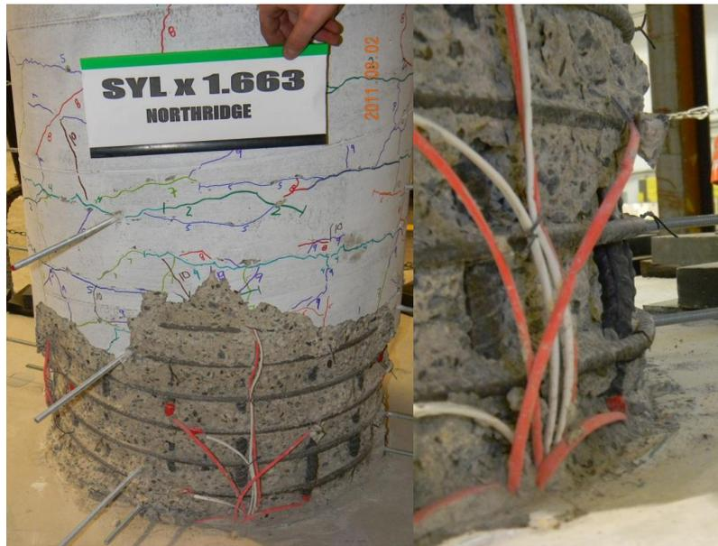
**Figure 4.3:** North Bent @ 350% of Design Earthquake
