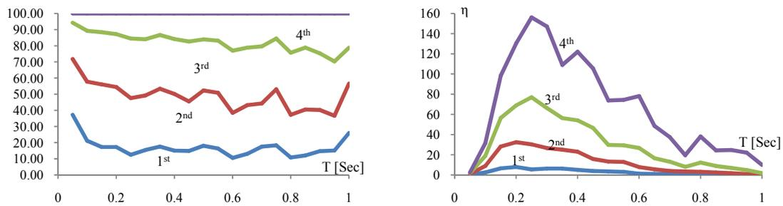
**Figure 4.5.** Energy Percentage Distribution and  $\eta$  for B Model under El Centro EW Earthquake
