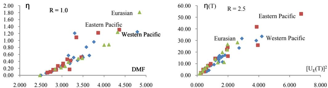
**Figure 2.2:** Cumulative Damage for  $R = 1$  and  $R = 2.5$  due to Various Earthquakes in the World
