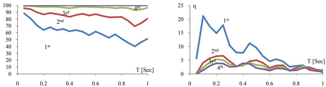
**Figure 4.3.** Energy Percentage Distribution and  $\eta$  for A Model under El Centro NS Earthquake
