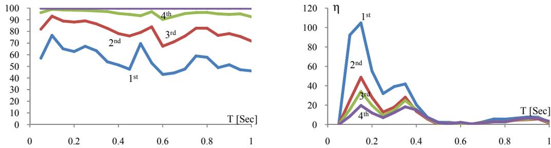
**Figure 4.4.** Energy Percentage Distribution and  $\eta$  for A Model under Hachinohe NS Earthquake
