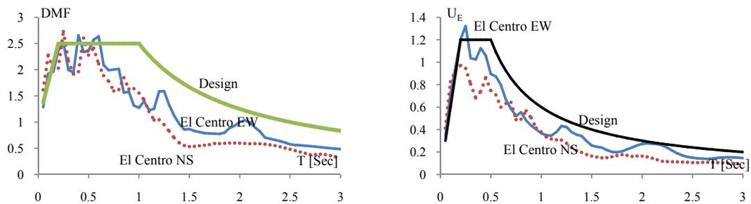
**Figure 2.1:** Dynamic Magnification Factor and Unit Acceleration
