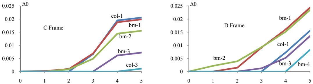
**Figure 4.8.** Plastic Hinge Rotation for Every Loading Stage Pushover Analysis
