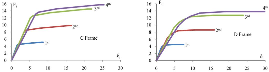
**Figure 4.7.** Load Deformation of C and D Frame Pushover analysis
