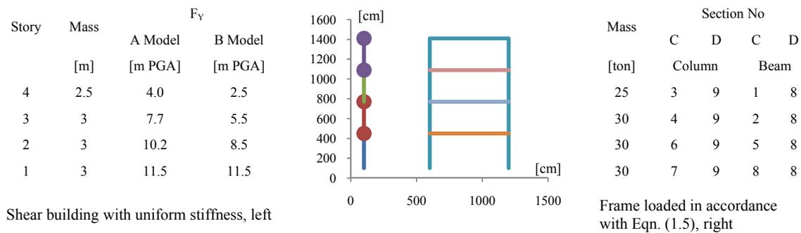
**Figure 4.1.** Four Story Shear Building and Frame Models
