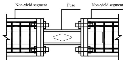
**Figure 3.1.** New coupling beams
