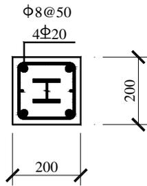
**Figure 3.4.** The reinforcement of non-yield segment
