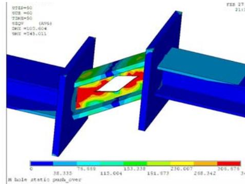
**Figure 4.6.** The von mises of "fuse"
