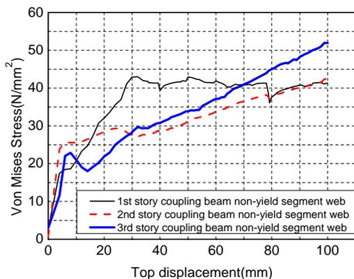
**Figure 4.13.** Von mises stress of non-yield segment web
