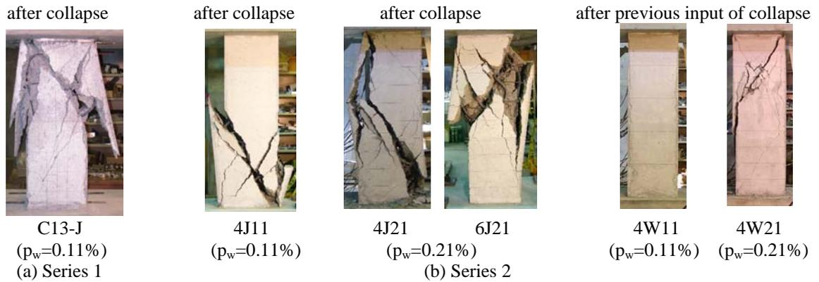
Figure 7. Damage states
