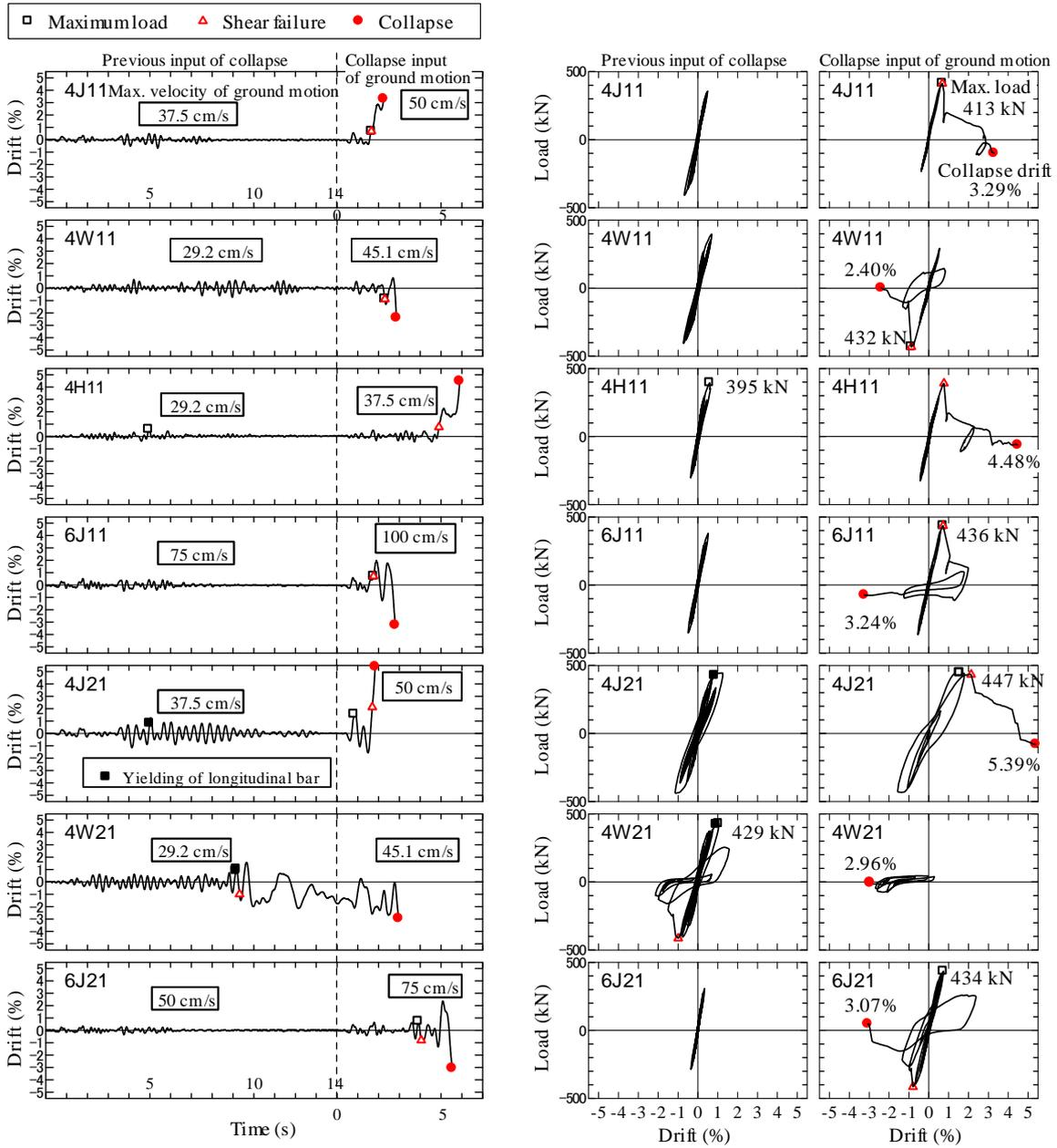
Figure 6. Time history of drift and lateral load vs. drift (series 2)
