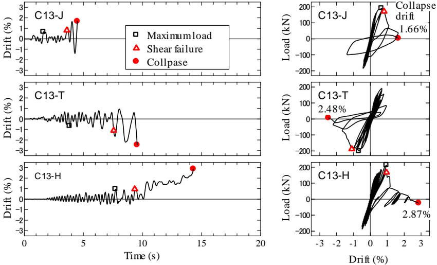
**Figure 5.** Time history of drift and lateral load vs. drift (series 1)
