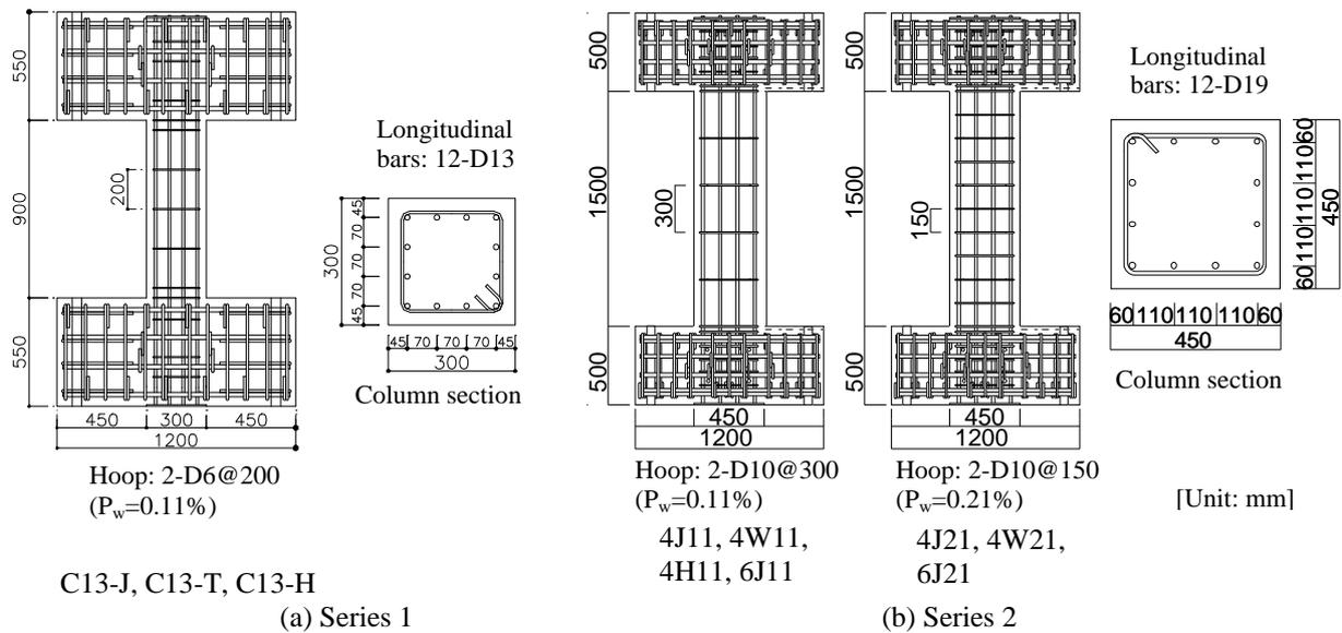
**Figure 2.** Reinforcement details of the specimens
