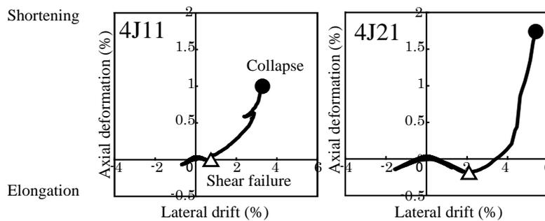
**Figure 12.** Lateral drift vs. axial deformation relations (specimens 4J11 and 4J21)
