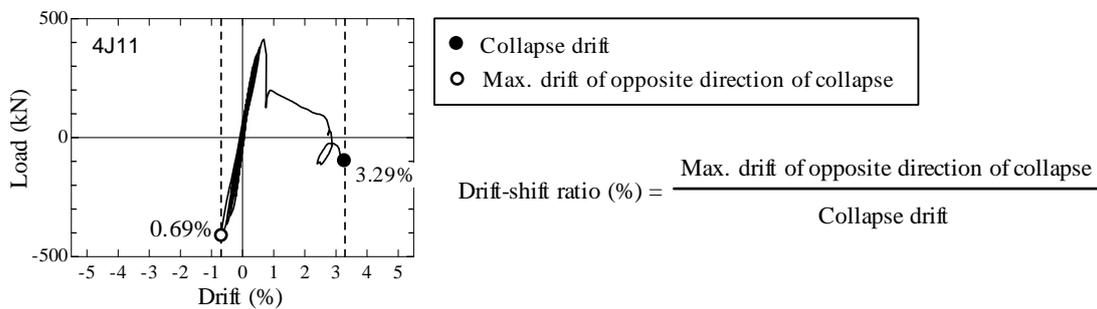
Figure 9. Evaluation of drift-shift ratio
