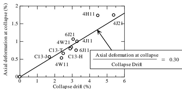
**Figure 13.** Axial deformation in collapse vs. collapse drift relations
