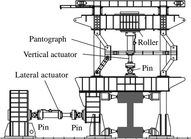
Figure 3. Test apparatus
