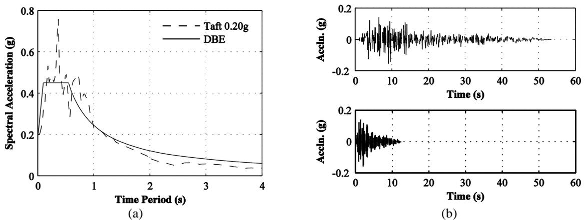
Figure 2.4. (a) Comparison of DBE for Zone V (PGA 0.18g) with Taft (PGA 0.20g) (b) Original and compressed Taft N21E ground motion
