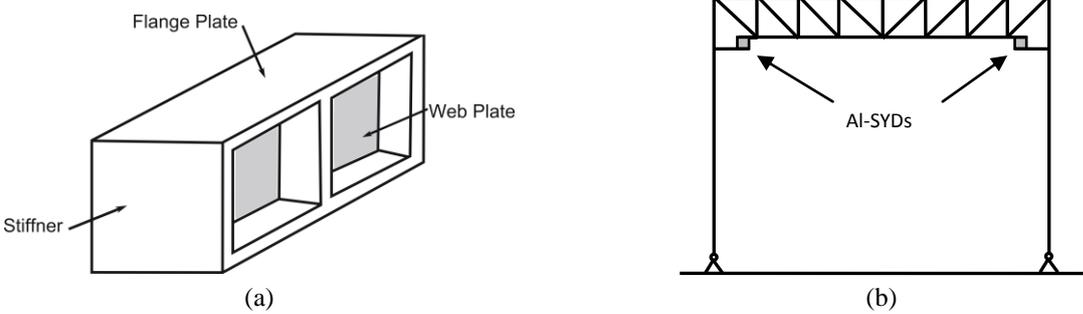
**Figure 1.1.** (a) Schematic diagram of typical Shear-link (b) Arrangement of Shear Link in Al-SYD TMF
