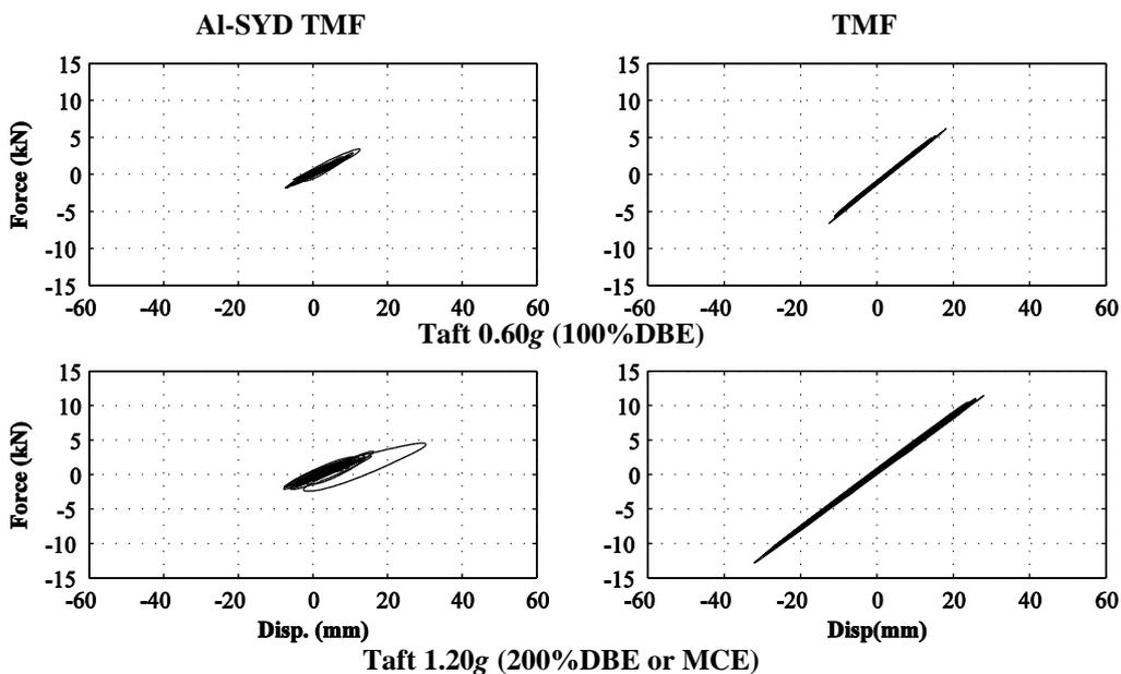
Figure 3.6. Hysteretic area plot for Al-SYD TMF and TMF at various PGA levels
