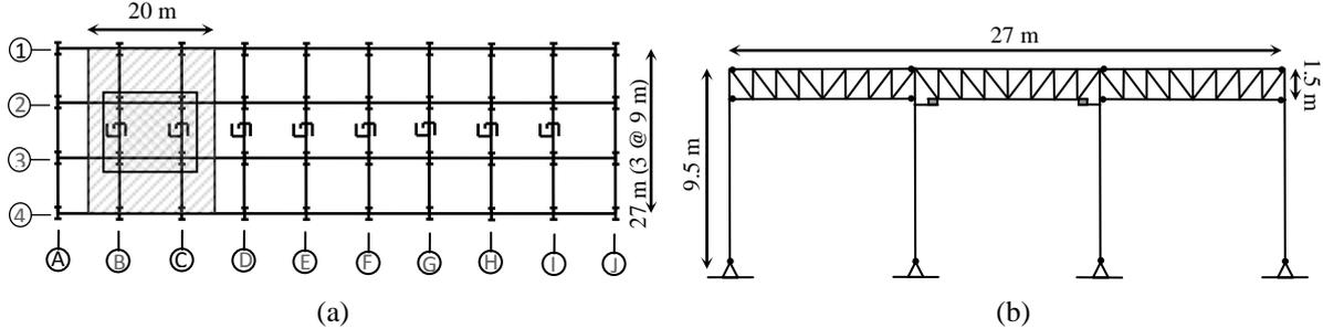
**Figure 2.1.** (a) Plan view of the prototype building and tributary area (b) Cross-sectional view of the frame
