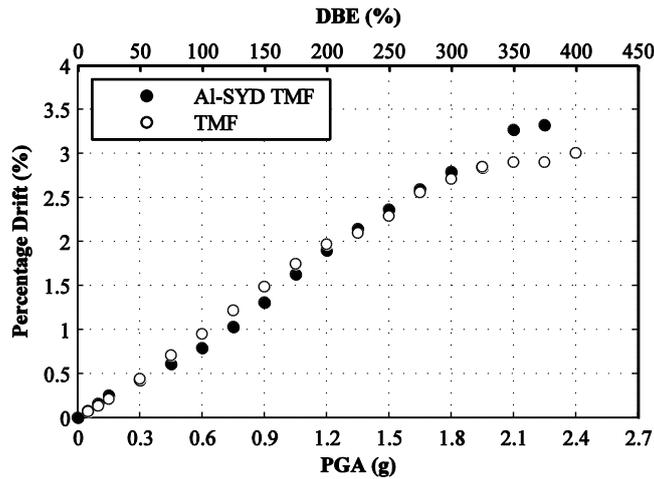
Figure 3.5. Comparison of maximum roof drift in Al-SYD and TMF at various DBE levels
