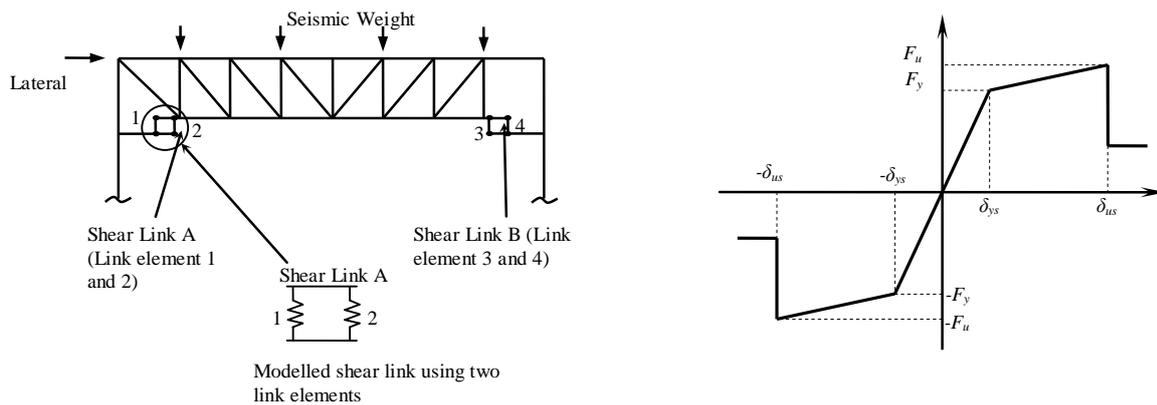
Figure 4.1. Modeling of shear link with multi-linear plastic element and backbone curve defined in SAP2000
