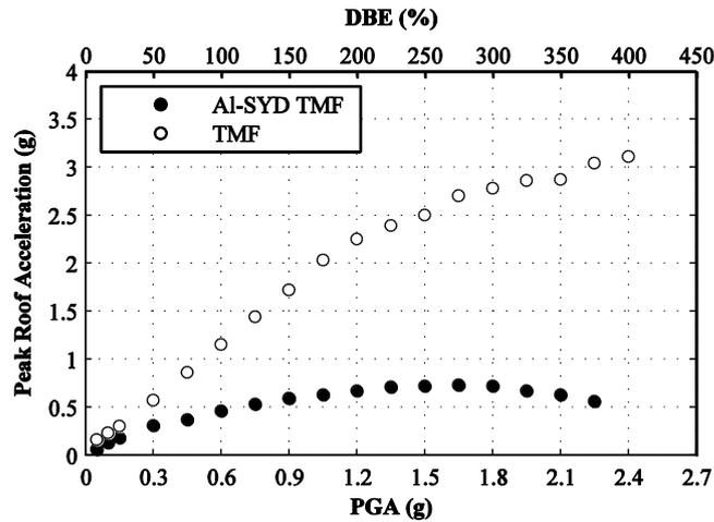
**Figure 3.3.** Comparison of peak roof acceleration experienced by Al-SYD TMF and TMF
