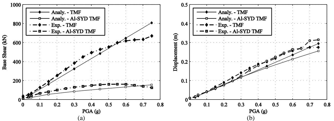
Figure 4.2. Base Shear and (b) Roof Displacement comparison between Analytical and Experimental analysis of TMF and AI-SYD TMF
