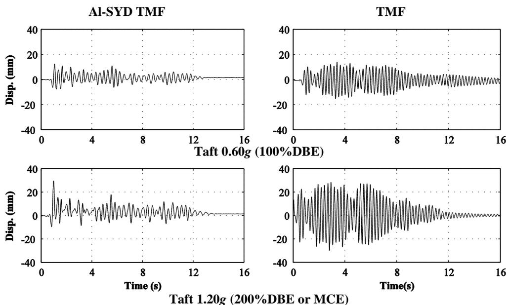
**Figure 3.4.** Displacement response comparison for different Taft Intensities
