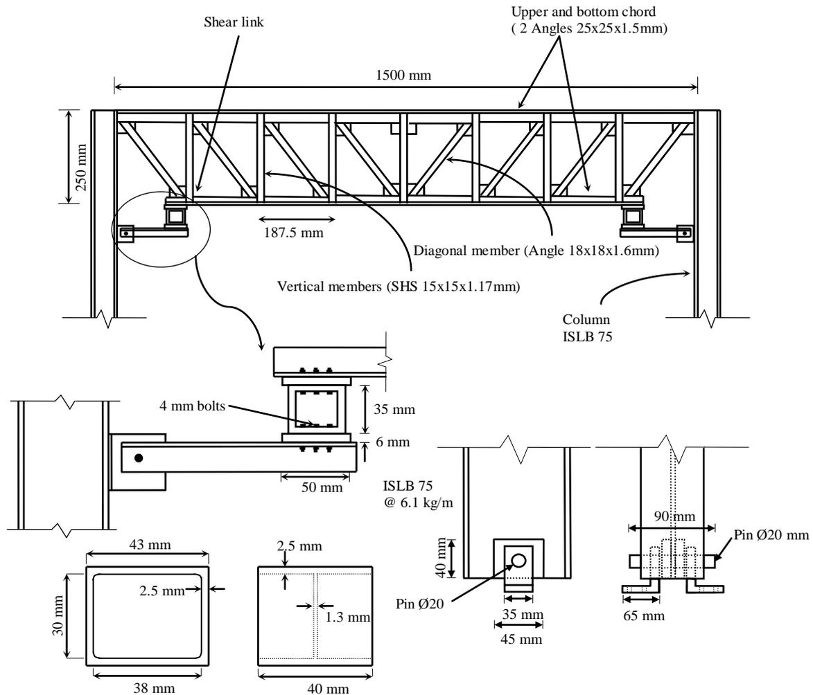
Figure 2.2. Schematic diagram of the shear link and model
