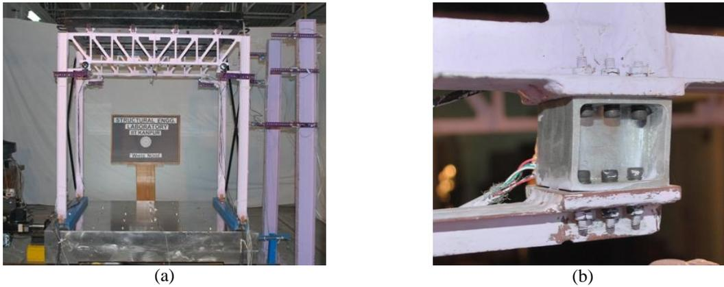
Figure 2.3. (a) Specimen mounted over the shake table (b) Arrangement of shear link in AI-SYD TMF
