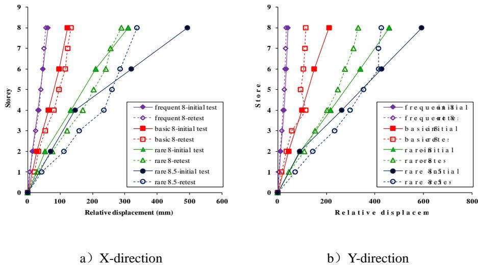
**Figure 7.** Comparisons of the maximum relative displacements of each storey of prototypes at different earthquake levels
