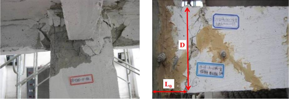
a) Joints failure of the model in initial test                      b) Joints failure of the model in retest
