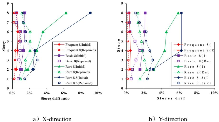
**Figure 8.** Comparisons of the maximum storey drift ratios of prototypes at different earthquake level
