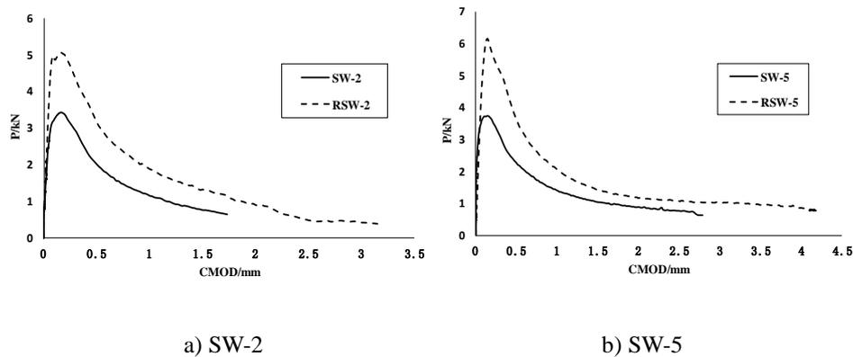
**Figure 1.** P-CMOD curves of specimens from initial test and retest
