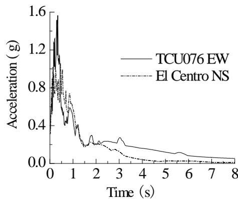
**Figure 3.2.** Response spectra of selected ground motions
