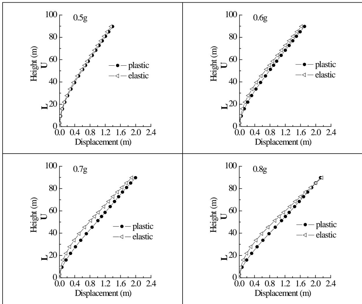
**Figure 5.5.** Comparison between deformed shape of pylon columns with and without the consideration of the nonlinear behavior of pylon
