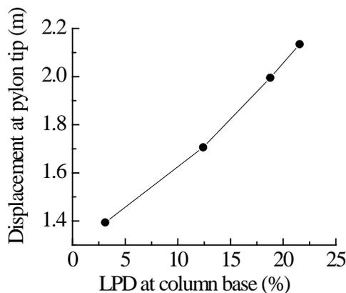
**Figure 5.4.** Relationship between level of plastic development at the column base and displacement at pylon tip
