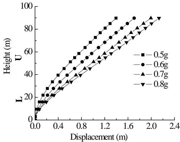
**Figure 5.1.** Deformation envelopes along the height of pylon columns with increment of PGA
