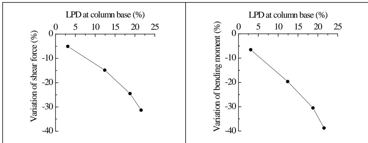
Figure 5.6. Effect of pylon yielding on the seismic induced force at the bottom of pylon pile cap
