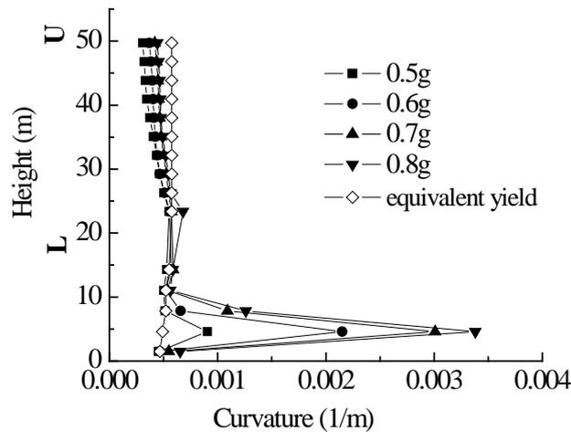
**Figure 5.2.** Curvature envelopes along the height of pylon columns with increment of PGA
