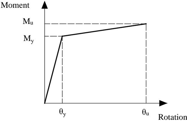
Figure 4.1. Typical bilinear curve of nonlinear link element
