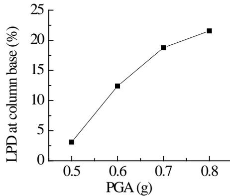
**Figure 5.3.** Variation trend of the level of plastic development at the column base with increment of PGA
