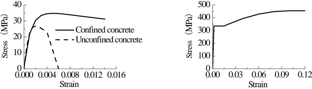
Figure 4.2. Material model of fiber hinge element
