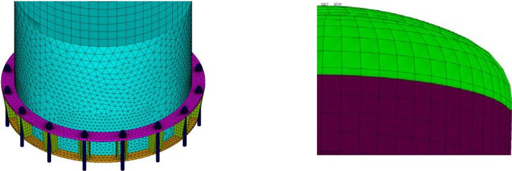
**Figure 2.4.** Lower segment at the level base of tower and the compression rings
