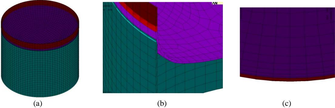
**Figure 2.3.** a. Steel skirt of tower b. Detail of the connection between the skirt and lower cap and c. Steel walls
