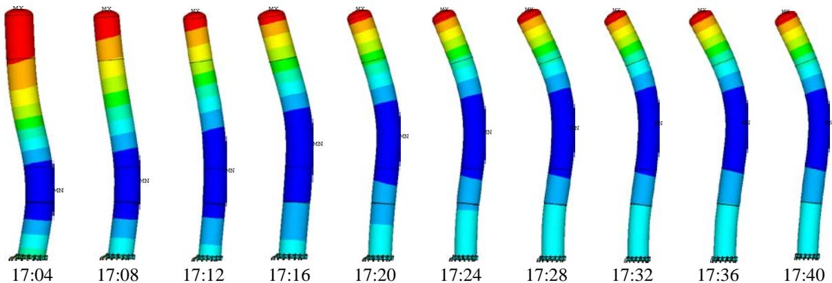
Figure 3.9. Sequence of the displacement of the tower for the 17:04 to 17:40 sec
