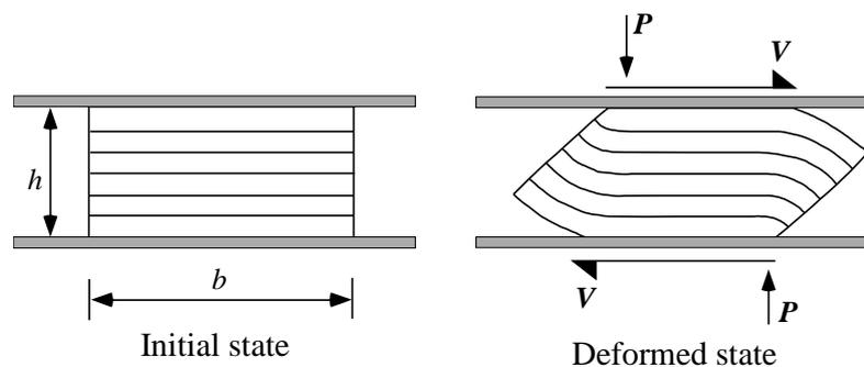
**Figure 4.1** Free body diagram of laterally deformed STRP isolator
