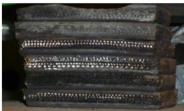
**Figure 2.1** Unbonded STRP-6 specimen isolator
