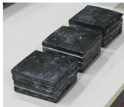
**Figure 2.2** Bonded STRP-4 specimens isolator
