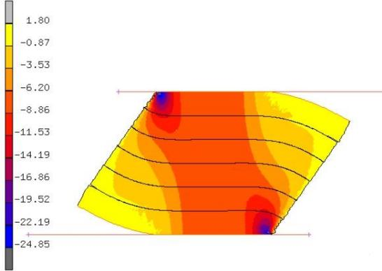
Fig. 4.2.3 Contour of normal stress  $S_{22}$  (MPa) in the rubber layers of the STRP-6 isolator
