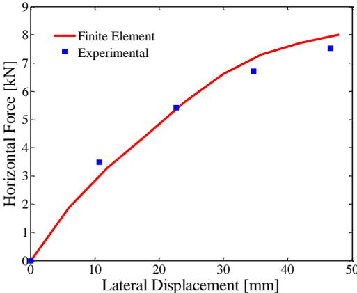
**Figure 4.2.1** Load-displacement relationships of STRP-6: comparison of experimental and FE analysis results
