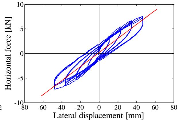
**Figure 3.3** Lateral load displacement relationship
