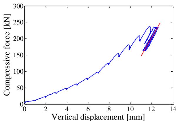
**Figure 3.4** Vertical load displacement relationship
