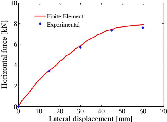
Figure 4.2.2 Load-displacement relationships of STRP-4: comparison of experimental and FE analysis results
