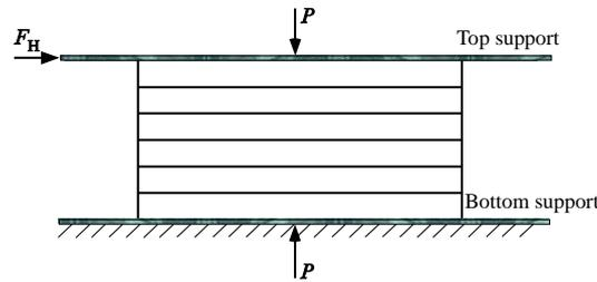
**Figure 3.1** Loading setup and boundary conditions
