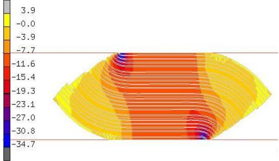
Fig. 4.2.4 Contour of normal stress  $S_{22}$  (MPa) in the rubber layers of the STRP-4 isolator
