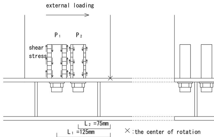
**Figure 4.4.** Analysis model for shear stress around lag screw bolts
