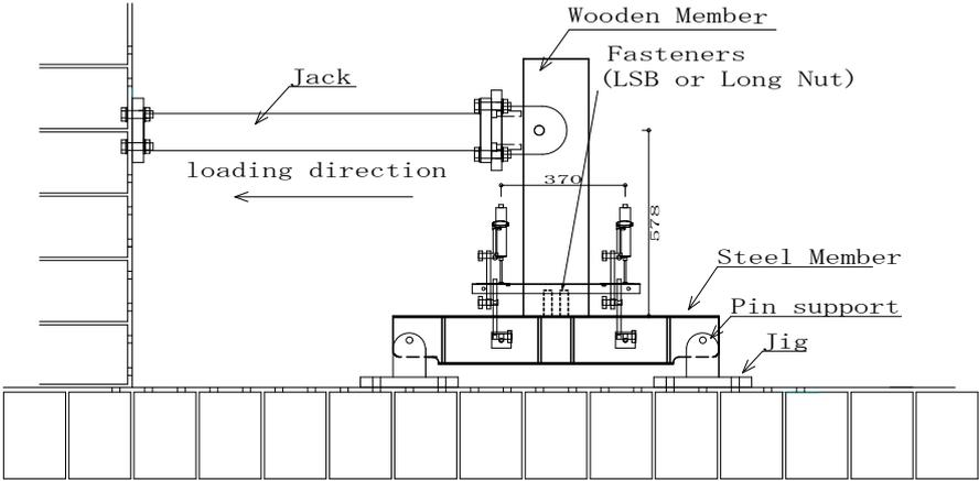
Figure 2.1. Setup of this test (Unit: mm)
