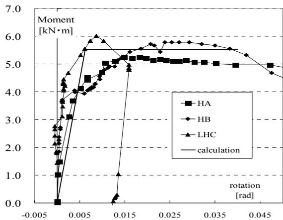
**Figure 3.9.** Moment-rotation curve (with 4 lag screw bolts)
