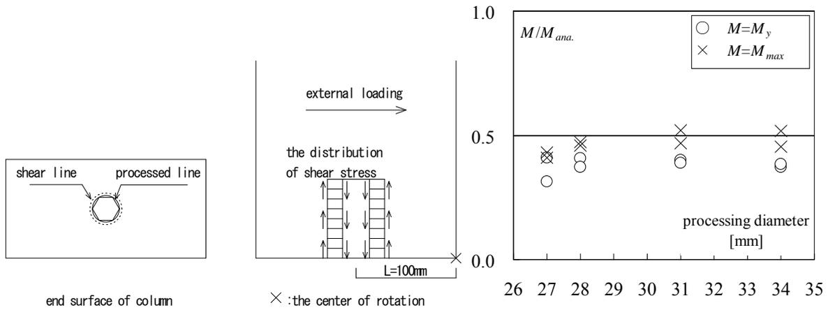
**Figure 4.1.** Analysis model of infill joint
