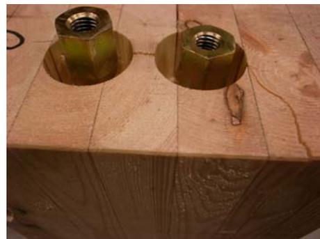
**Figure 3.6.** Pulled out of lag screw bolt
