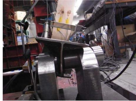
**Figure 3.8.** Out-plane buckling (LHC)
