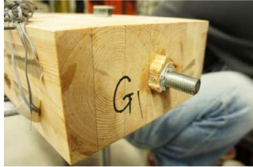
**Figure 3.4.** Pulled out of infill joint
