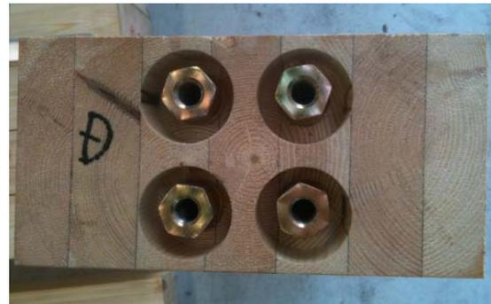
**Figure 2.5.** Inserted condition of lag screw bolt
