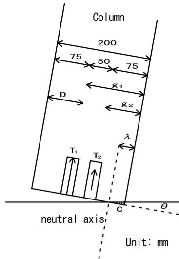
**Figure 4.3.** Analysis model for pulling out of lag screw bolts
