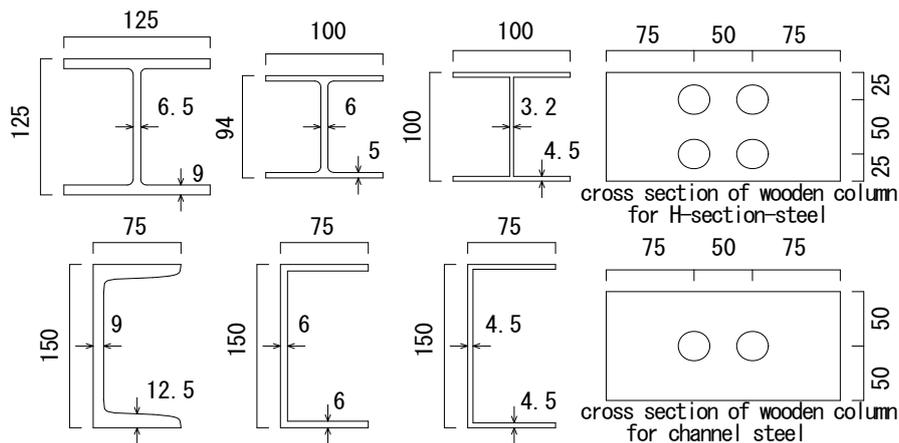
**Figure 2.6.** The dimension of each members and the arrangement of lag screw bolt (Unit: mm)
