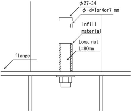
Figure 2.2. Pattern diagram of infill joint.
