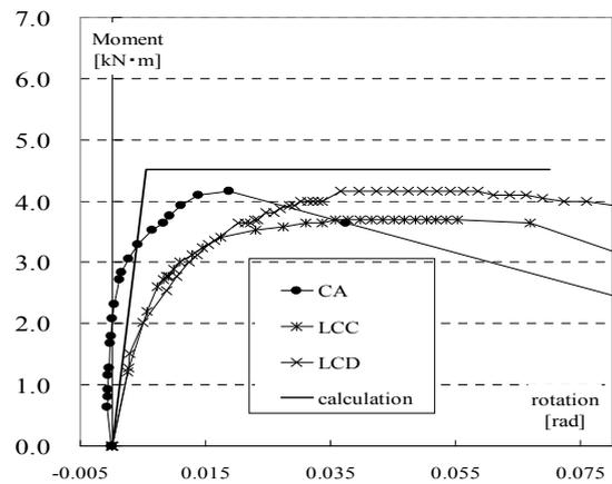
**Figure 3.10.** Moment-rotation curve (with 2 lag screw bolts)
