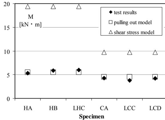
**Figure 4.5.** Analysis results of LSB joints
